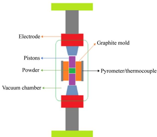
Fig.3 Schematic diagram of SPS equipment
