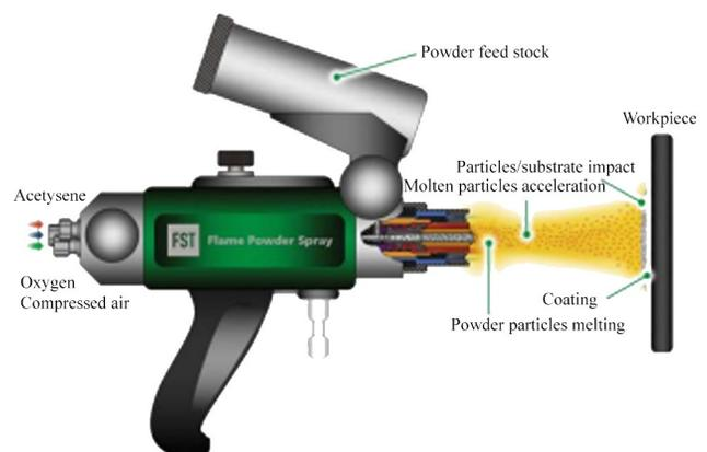
Fig.5 Schematic diagram of TSP method<sup>[60]</sup>
