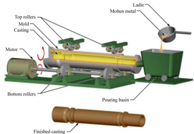
Fig.7 Schematic diagram of CCP<sup>[66]</sup>
