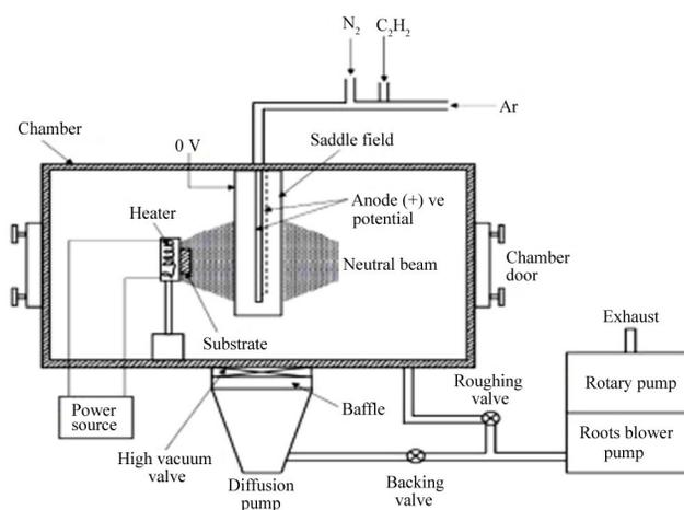
Fig.6 Schematic diagram of low-temperature plasma nitriding process<sup>[65]</sup>
