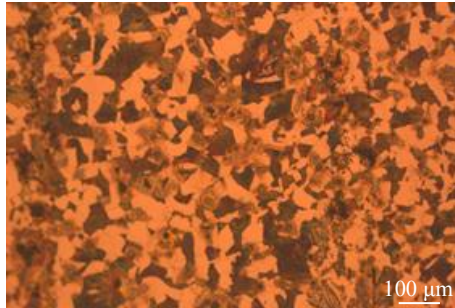
Fig.2 Microstructure of 20CrNiMo steel substrate
