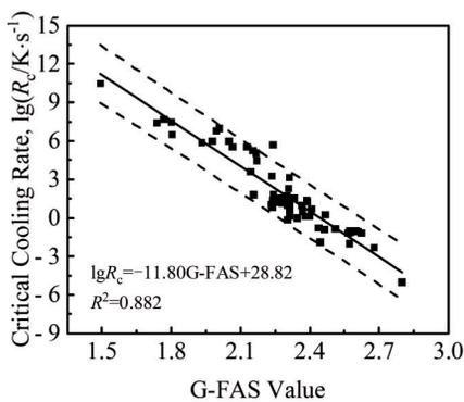
Fig.3 Correlation between G-FAS criterion and critical cooling rate  $\lg R_c$  of various metallic glasses
