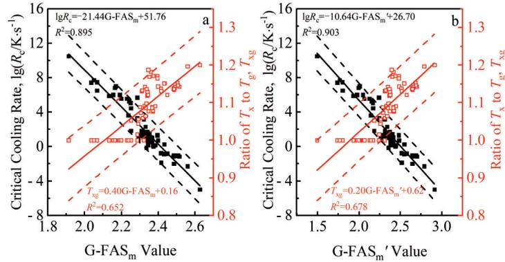
Fig.5 Correlations of modified G-FAS<sub>m</sub> criterion (a) and G-FAS<sub>m</sub>' criterion (b) with critical cooling rate  $R_c$  and the ratio of  $T_x/T_g$  ( $T_{xg}$ ) for various metallic glasses
