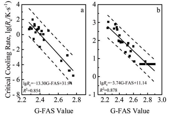
Fig.4 Correlations between G-FAS criterion and critical cooling rate  $\lg R_c$  of 23 glassy oxides (a) and 31 cryoprotective solutions (b)
