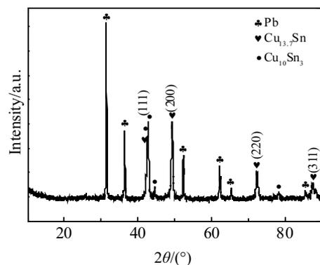
Fig.4 XRD pattern of as-cast 14Sn-64.5Cu-21.5Pb (wt %) alloy
