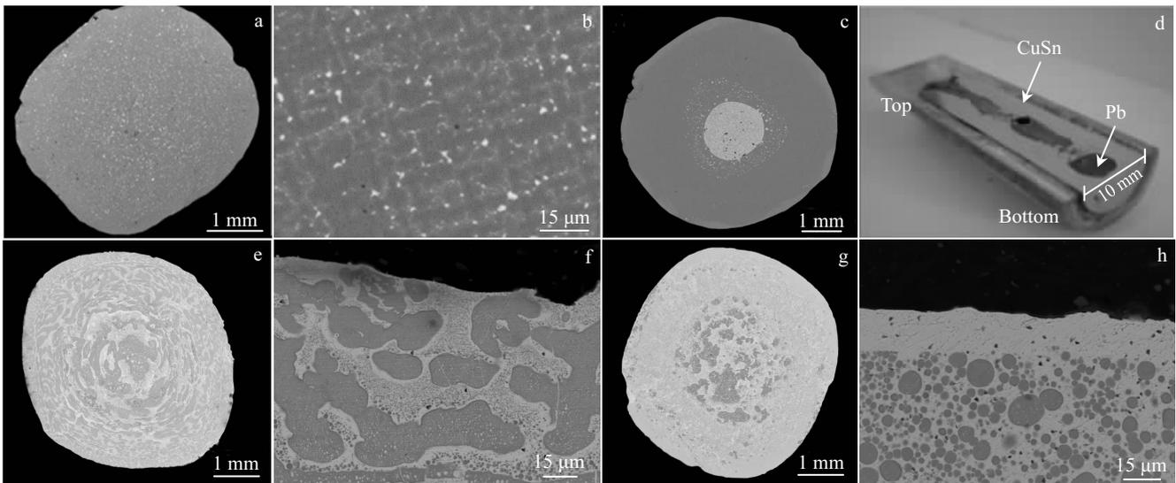
Fig.2 Cross-sectional morphologies of as-cast 14Sn-73.1Cu-12.9Pb alloy (a) and its partial enlarged detail (b); 14Sn-64.5Cu-21.5Pb alloy (c) and its axial direction cross-sectional morphology (d); Cu-65Pb alloy (e) and its enlarged boundary (f); Cu-75Pb alloy (g) and its enlarged boundary (h)
