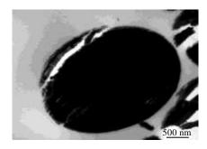
图 4 CTAB 为活性剂时制备的 SnO<sub>2</sub> 实心微球截面 TEM 照片 Fig.4 TEM image of cross-section of SnO<sub>2</sub> solid microsphere using CTAB as surfactant
