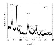
图 5 CTAB 为活性剂时制备的 SnO<sub>2</sub> 实心微球 XRD 图谱 Fig.5 XRD pattern of SnO<sub>2</sub> solid microsphere using CTAB as surfactant
