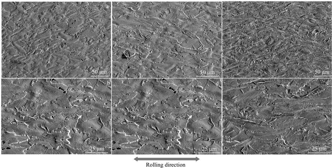
Fig.4 SEM images of the GNPs/Ti composites at different rolling reductions: (a, b) 20%, (c, d) 40%, and (e, f) 60%
