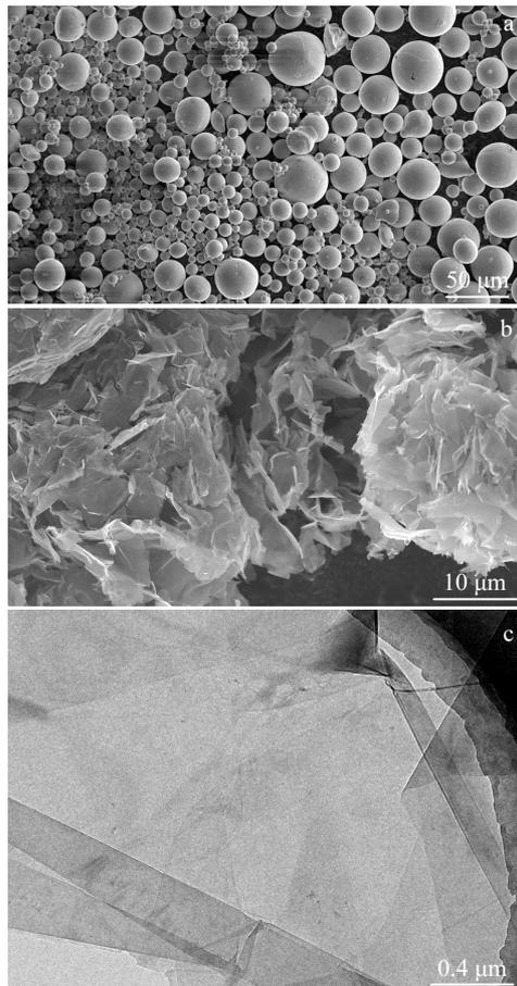
Fig.1 SEM (a, b) and TEM (c) images of initial powder: (a) Ti powder and (b, c) GNPs powder
