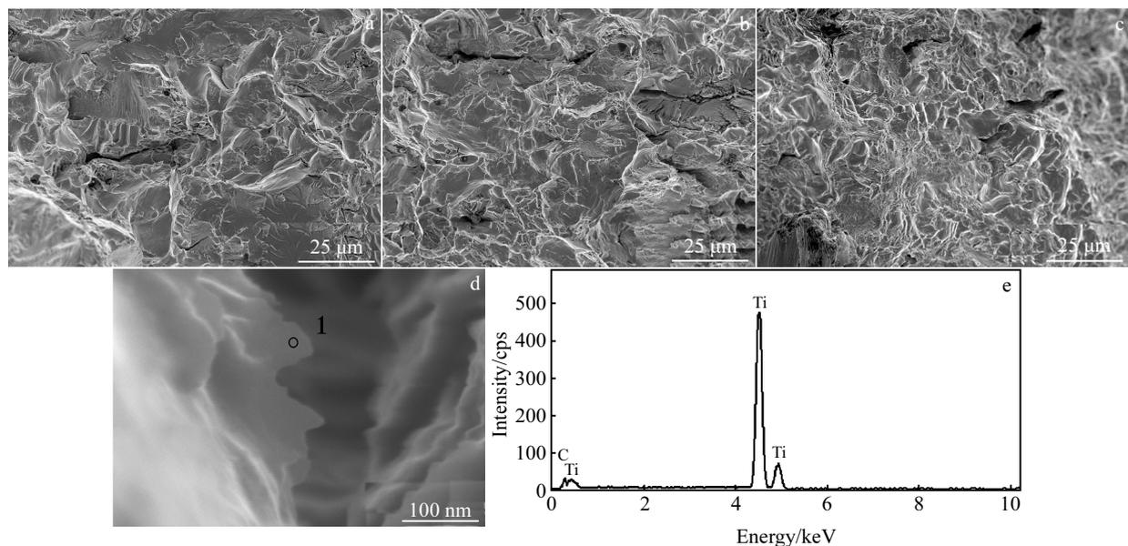
Fig.5 SEM fracture surfaces (a~c) and EDS spectrum of point 1 (d,e) for GNPs/Ti composite: (a) 20%, (b) 40%, and (c) 60%
