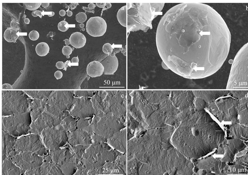
Fig.3 SEM images of the mixed powder and sintered composite: (a,b) mixed powder and (c,d) sintered GNPs/Ti composite
