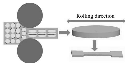
Fig.2 Diagram of the rolling process and sampling
