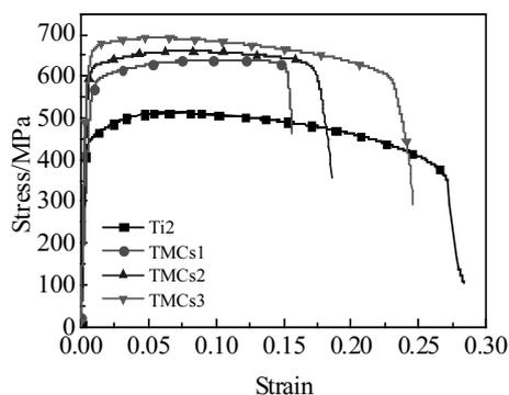
Fig.6 Room temperature tensile properties of specimens hot-rolled at different reductions
