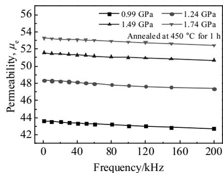
Fig.6 Permeability ( $\mu_e$ ) of the  $\text{Fe}_{95}\text{Si}_1\text{B}_2\text{P}_{0.5}\text{Cu}_{1.5}$  magnetic powder core formed at different pressures
