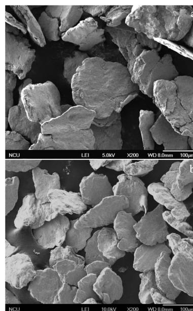
Fig.1 SEM images of  $\text{Fe}_{95}\text{Si}_1\text{B}_2\text{P}_{0.5}\text{Cu}_{1.5}$  alloy powders: (a) 75~150  $\mu\text{m}$  and (b) 45~75  $\mu\text{m}$
