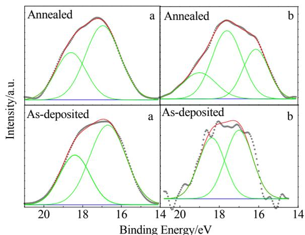
Fig.1 Hf4f spectra for the as-deposited film and the annealed film, respectively: (a) with a blocking layer, (b) without blocking layer
