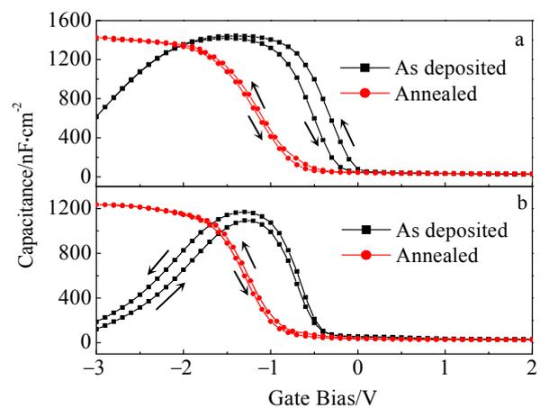
Fig.5 Capacitance characteristics of MIS capacitors made of the as-deposited film and the annealed film, respectively: (a) with a blocking layer, (b) without blocking layer
