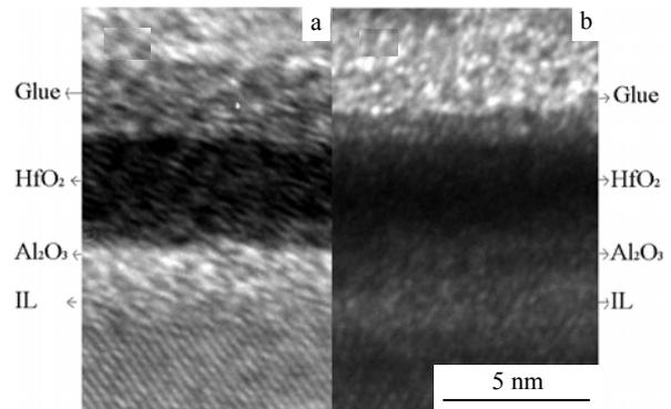
Fig.4 HRTEM images for the samples with blocking layer: (a) annealed and (b) as-deposited
