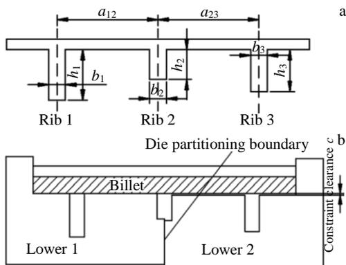
Fig.1 Eigenstructure and its local loading process: (a) geometry and (b) local loading process
