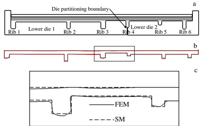
Fig.4 Local loading process of multi-ribs: (a) FE model, (b) shape of multi-ribs after two local loading steps, and (c) shape in enlarging area
