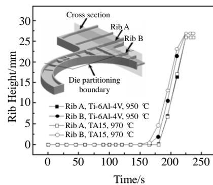
Fig.5 Rib heights on the cross section in the local loading process by using different materials (FEM result)
