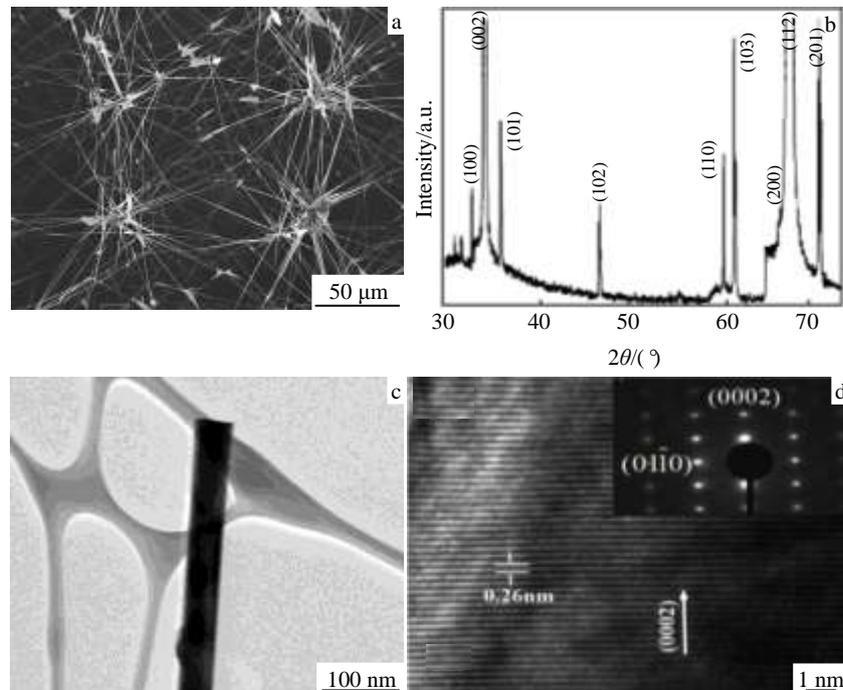
Fig.1 Characterization results for the as-synthesized ZnO nanowire network on the edge of the columnar electrode: (a) SEM image of ZnO nanowire network, (b) XRD pattern of the as-grown nanowires, (c) TEM image of a typical nanowire, and (d) high resolution TEM image of nanowire. (inset is the corresponding TEM diffraction pattern)
