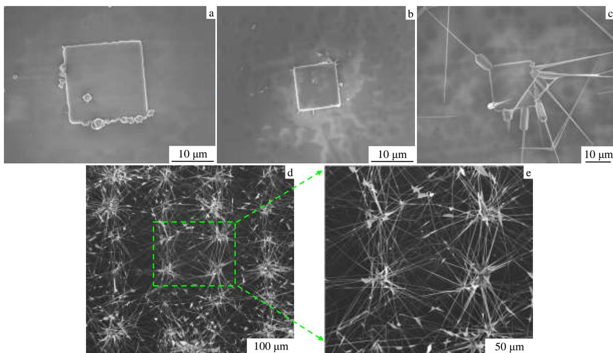
Fig.2 SEM images of ZnO nanowires grown on a bare silicon substrate with cylindrical electrodes: (a-c) growth result with a synthesis time of 10, 20 min; (d) low magnification SEM image of the growth result with a synthesis time of 30 min; (e) zoom in SEM image of the area with the red line indicated in Fig.2d
