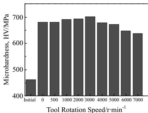
Fig.7 Micro-hardness values of AA7075-O formed parts at various rotation speeds
