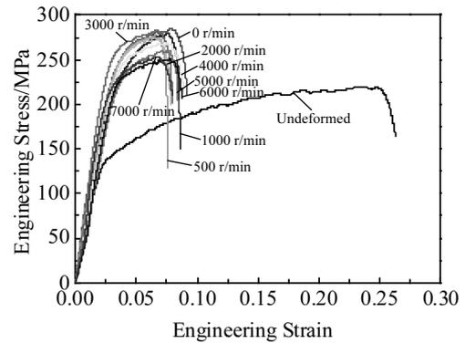
Fig.8 Engineering stress-strain curves of AA7075-O sheets at various rotation speeds
