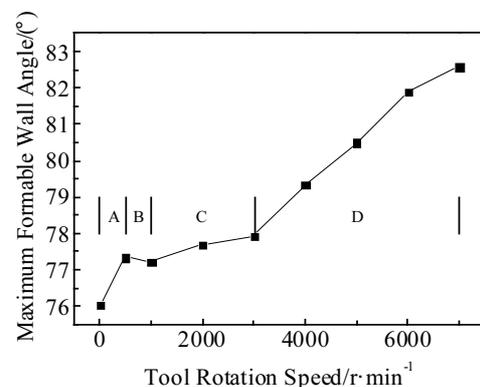
Fig.3 Formability at different tool rotation speeds
