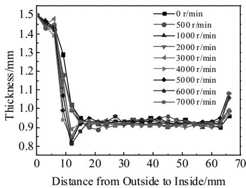
Fig.9 Thickness distribution of parts formed at different rotation speeds
