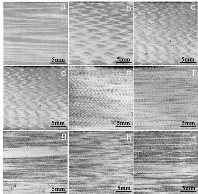
Fig.5 Surface topography of parts formed at different rotation speeds: (a) 0 r/min, (b) 500 r/min, (c) 1000 r/min, (d) 2000 r/min, (e) 3000 r/min, (f) 4000 r/min, (g) 5000 r/min, (h) 6000 r/min, and (i) 7000 r/min
