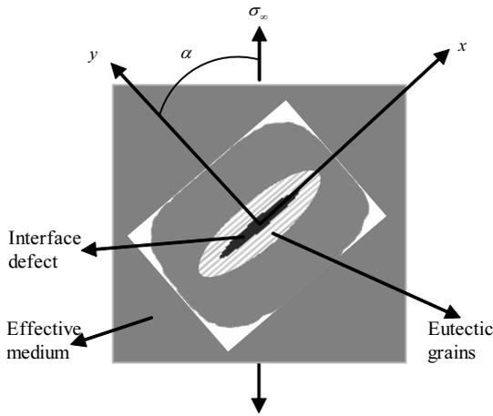
Fig.3 A meso-cell embedded in the equivalent medium
