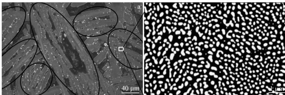
Fig.1 SEM Microstructures of the ceramic composites in different scales<sup>[28]</sup>: (a) eutectic composite ceramic and (b) rod-shaped eutectic grains with fibers
