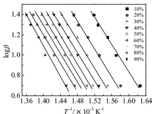
Fig.2 Ozawa plots of  $\log\beta$  versus  $T^{-1}$  at different heating rates ( $\beta$ ) for compound  $\text{Ba}(\text{DPM})_2$
