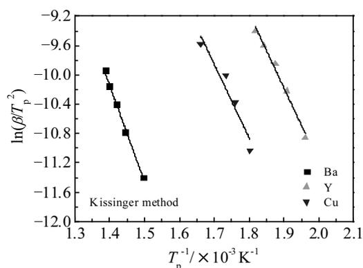
Fig.6 Kissinger plots of  $\ln(\beta/T_p^2)$  versus  $T_p^{-1}$  at different heating rates ( $\beta$ ) for compound  $\text{Ba(DPM)}_2$ ,  $\text{Y(DPM)}_3$ , and  $\text{Cu(DPM)}_2$
