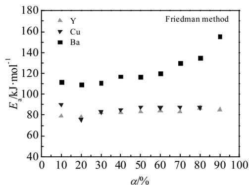
Fig.5 Apparent activation energy ( $E_a$ ) versus different extents of conversion ( $\alpha$ ) by Friedman method for compound  $\text{Ba(DPM)}_2$ ,  $\text{Y(DPM)}_3$ , and  $\text{Cu(DPM)}_2$
