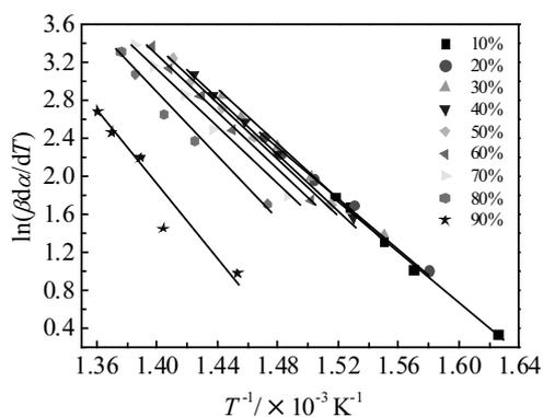
Fig.4 Friedman plot of  $\ln(\beta da/dT)$  versus  $T^{-1}$  at different heating rates ( $\beta$ ) for compound  $\text{Ba(DPM)}_2$
