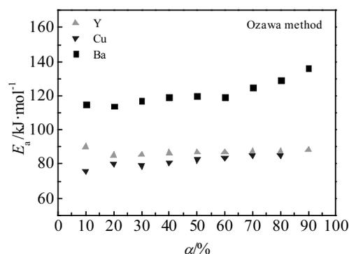
Fig.3 Apparent activation energy ( $E_a$ ) versus different extents of conversion ( $\alpha$ ) by Ozawa method for compound  $\text{Ba}(\text{DPM})_2$ ,  $\text{Y}(\text{DPM})_3$ , and  $\text{Cu}(\text{DPM})_2$
