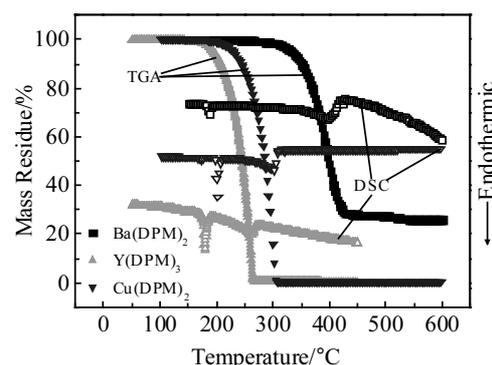
Fig.1 Ambient pressure TGA and DSC of  $\text{Y}(\text{DPM})_3$ ,  $\text{Cu}(\text{DPM})_2$  and  $\text{Ba}(\text{DPM})_2$  at a heating rate of 10 °C/min under a nitrogen atmosphere at a flow rate of 100 mL/min
