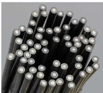
Fig.3 Morphology of flux-cored brazing filler metal
