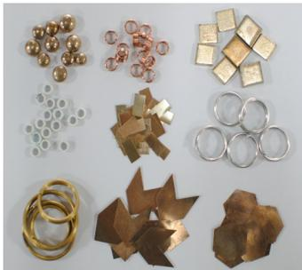
Fig.4 Morphology of the preformed filler metal
