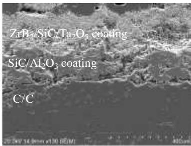
Fig.7 SEM image of the cross section of coating
