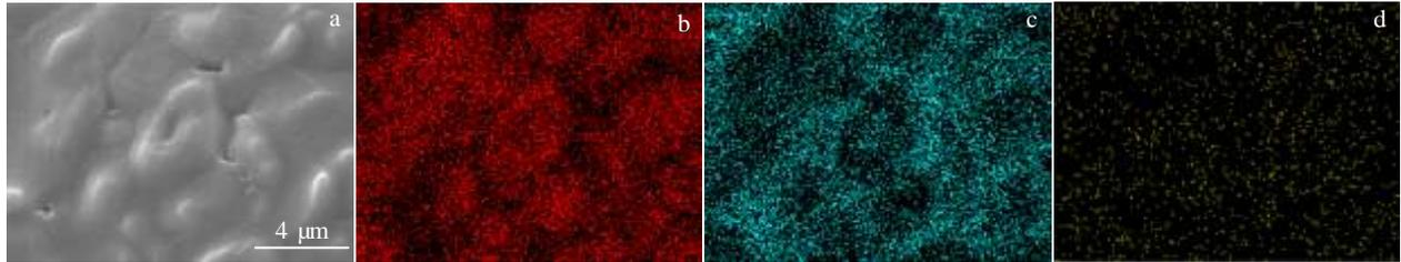
Fig.11 Morphology of center region after ablation for 30 s (a) and elements distribution of Zr (b), Si (c), and Ta (d)
