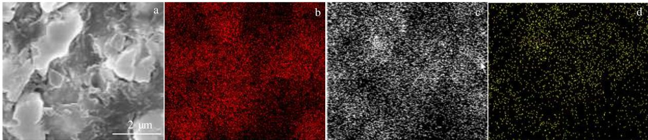
Fig.8 Morphology of cross section of  $ZrB_2/SiC-Ta_2O_5$  coating (a) and elements distribution of Zr (b), Si (c), and Ta (d)
