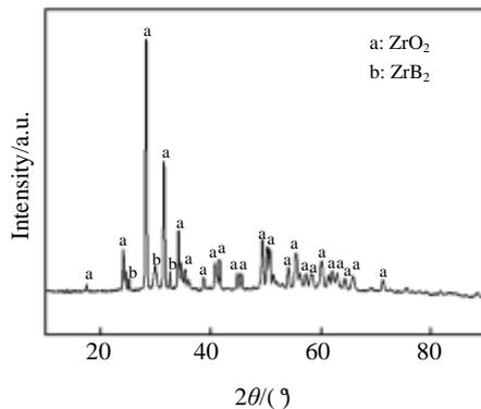
Fig.9 XRD pattern of the coating after ablation
