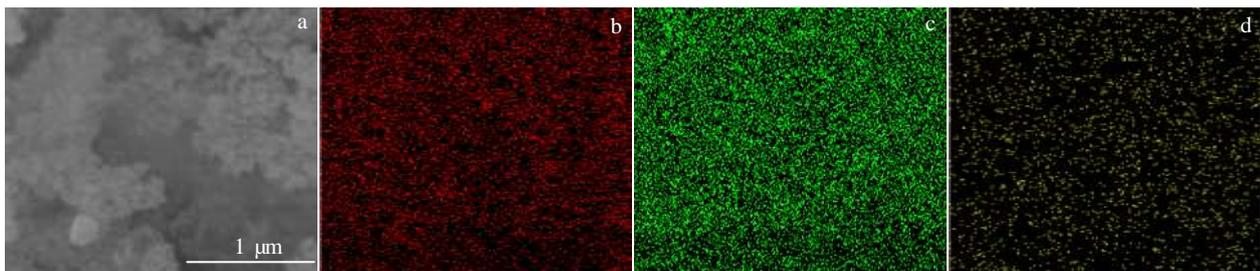
Fig.6 Morphology of coating surface (a) and element distribution of Zr (b), Si (c), and Ta (d)
