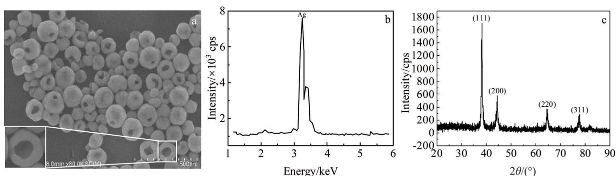
Fig.1 SEM morphology (a), EDS spectrum (b), and XRD pattern (c) of Ag nanobowls
