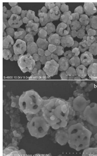
Fig.5 SEM morphologies of Ag nanobowls produced by reductant C<sub>6</sub>H<sub>8</sub>O<sub>6</sub> (a) and NaBH<sub>4</sub> (b)
