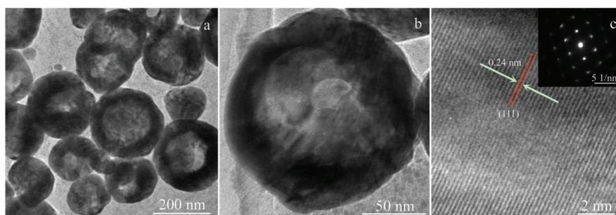
Fig.2 TEM images of Ag nanobowls (a, b); HRTEM image and SAED pattern of the shell of Ag nanobowls (c)
