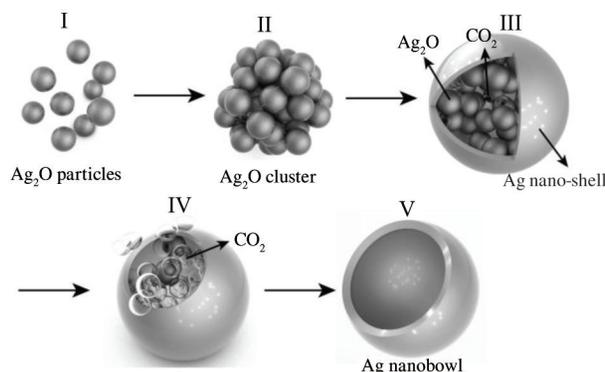
Fig.6 Schematic diagram of growth mechanism of Ag nanobowls
