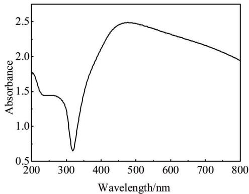
Fig.7 UV-visible spectrum of Ag nanobowls
