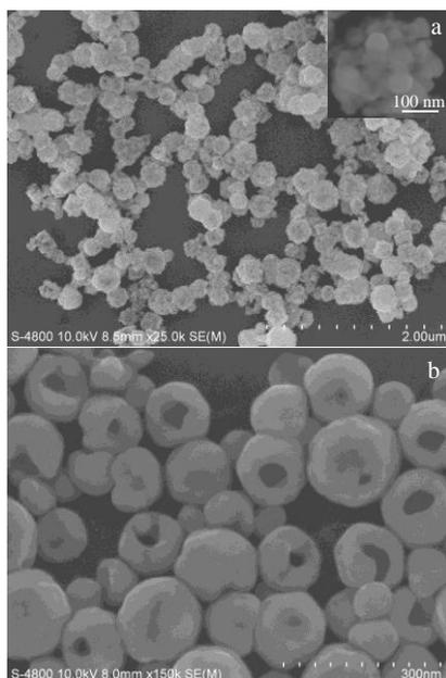
Fig.4 SEM morphologies of Ag<sub>2</sub>O nanoparticles before (a) and after (b) CH<sub>2</sub>O addition
