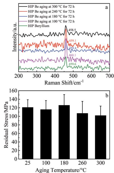
Fig.2 Residual stress of HIP beryllium after different low-temperature aging: (a) Raman method and (b) nano indentation method
