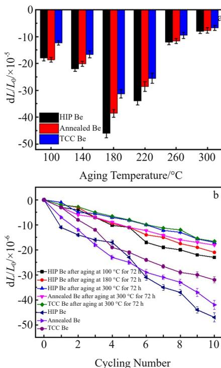
Fig.1 Dimensional changes of beryllium during aging in the range of 100–300 °C (a) and thermal cycles (b)
