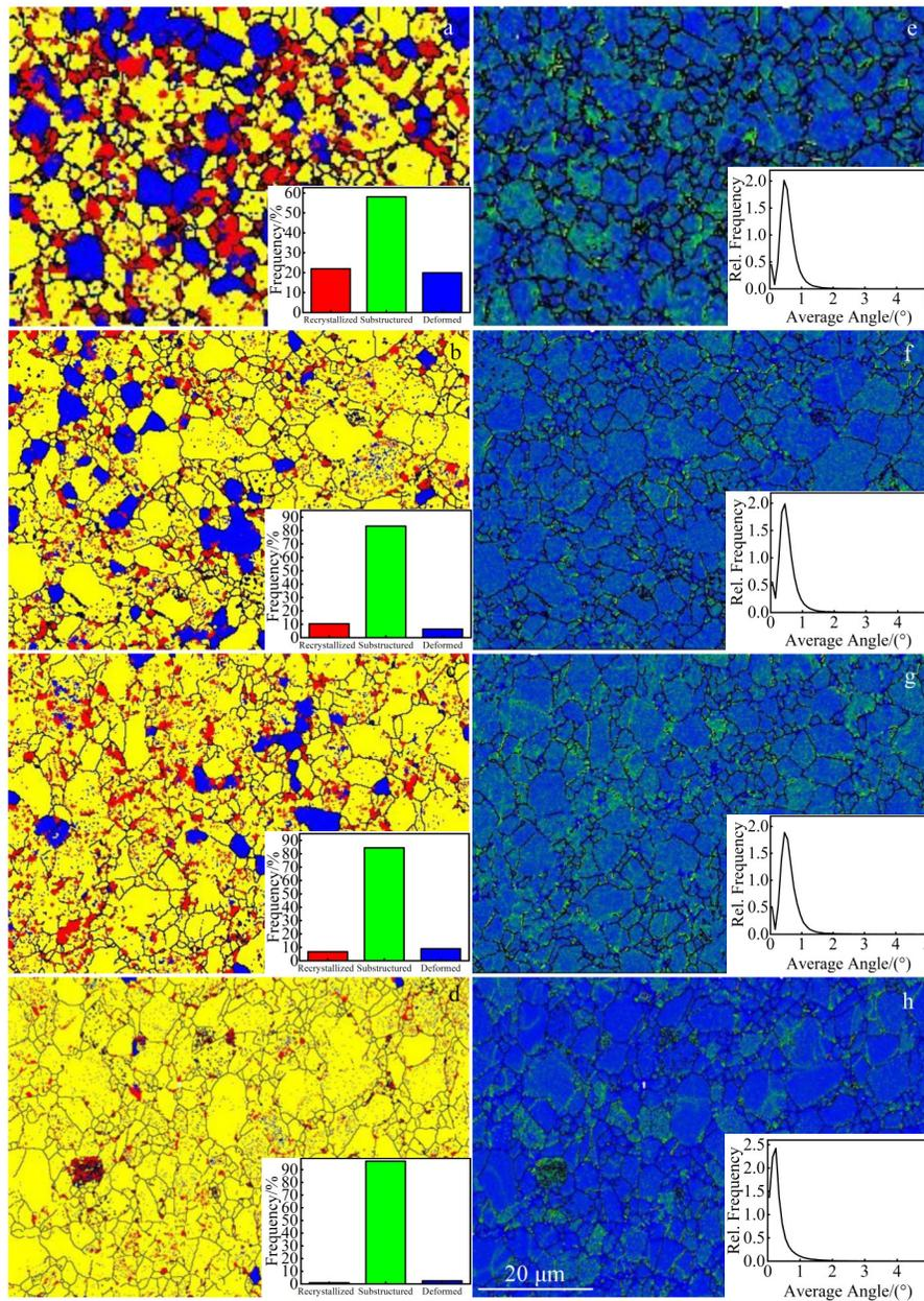
Fig.3 Misorientations (a–d) and dislocation density (e–h) of HIP beryllium: (a, e) before aging, (b, f) aging at 100 °C, (c, g) aging at 180 °C, and (d, h) aging at 300 °C
