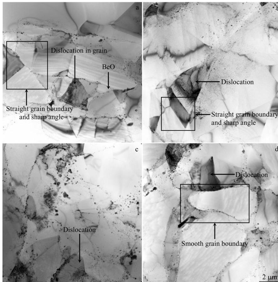
Fig.4 TEM images of HIP beryllium after different low-temperature aging: (a) before aging, (b) aging at 100 °C, (c) aging at 180 °C, and (d) aging at 300 °C
