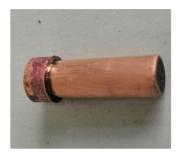
Fig.10 Real photograph of Cu/NbTi sample after cladding extrusion
