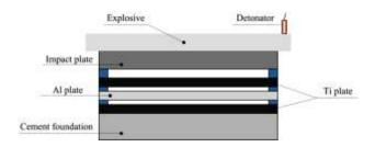
Fig.1 Explosive cladding experiment of Ti/Al/Ti laminate composites
