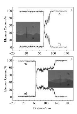
Fig.3 EDX line scanning analysis results of the interface: (a) the first layer and (b) the second layer
