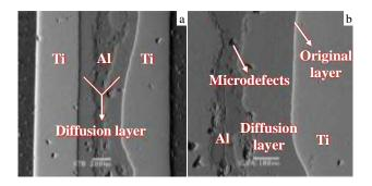
Fig.4 SEM images of Ti/Al/Ti laminates after heat treatment
