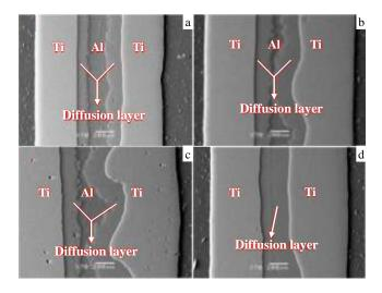
Fig.6 SEM images of Ti/Al/Ti laminates after hot pressing at 650 °C for different time: (a) 1 h, (b) 1.5 h, (c) 2 h, and (d) 2.5 h
