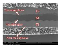
Fig.2 Bonding interface of Ti/Al/Ti laminate composites
