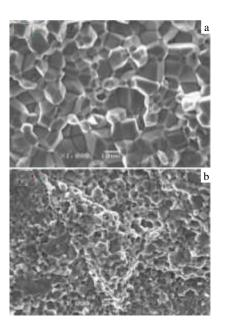
Fig.9 Fracture morphologies of diffusion layer after hot pressing for 2.5 h (a) and 3 h (b)
