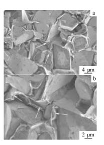
Fig.8 Surface morphology of fractured WC-Ni composite
