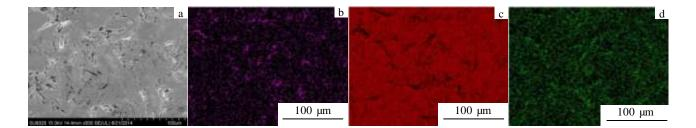
Fig.4 SEM image (a) and EDS map of the sample with Ni (3wt%) after sintering: (b) Ni, (c) W, and (d) C
