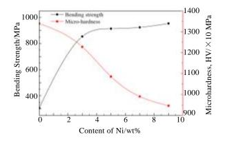
Fig.6 Bending strength and micro-hardness curves of the coated specimens with different Ni contents
