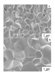
Fig.7 Surface morphology of fractured pure WC sample
