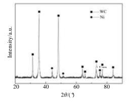
Fig.5 XRD pattern of the WC-9wt% Ni composites
