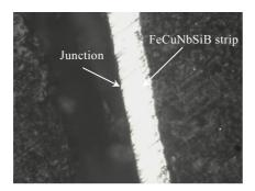
Fig.7 Microstructure of FeCuNbSiB amorphous alloy strips/ epoxy resin composite
