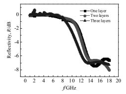
Fig.11 Effect of layer number on reflectivity of composites materials
