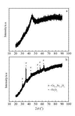
Fig.6 XRD patterns of strips before (a) and after (b) modification
