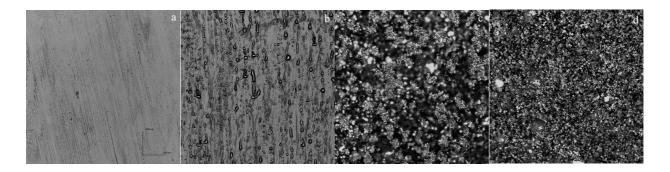
Fig.3 Surface morphologies of the strips before and after surface chemical modification: (a) free side of untreated strip; (b) roll side of untreated strip; (c) free side of modification strip; (d) roll side of modification strip
