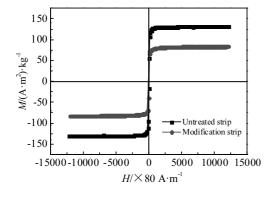
Fig.8 Hysteresis loops of amorphous alloy strips
