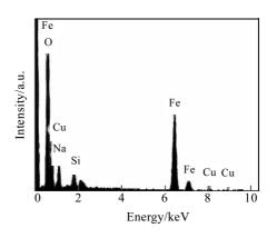
Fig.5 EDS spectrum of the strip conversion coat
