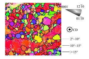
Fig.3 Orientation map of Mg-1Zn-1Gd alloy deformed after extrusion to 4 passes
