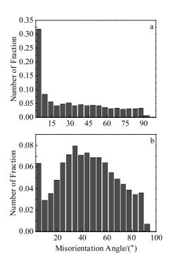
Fig.8 Misorientation angle distributions after 4 passes (a) and 8 passes (b)
