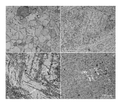
Fig.2 Microstructural evolution of Mg-1Zn-1Gd alloy after ECAP at 350 °C with a rate of 12 mm/min: (a) as-cast, (b) 1 pass, (c) 4 passes, and (d) 8 passes
