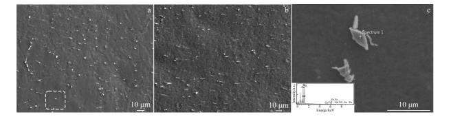
Fig.4 SEM images of Mg-1Zn-1Gd alloy deformed in extrusion to 4 passes (a) and 8 passes (b); (c) particles and EDS results of point marked in Fig.4a
