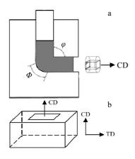
Fig.1 Schematic diagram of equal channel angular pressing (a) and sample in transverse direction (TD) and compressing direction (CD) (b)
