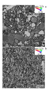
Fig.6 EBSD maps of Mg-1Zn-1Gd alloy after 4 passes (a) and 8 passes (b)
