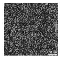
Fig.5 EBSD results of Mg-1Zn-1Gd at extrusion 8 passes corresponding TO boundary misorientation map
