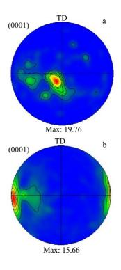
Fig.7 (0001) pole figures of dynamic recrystallized grains after 4 passes (a) and 8 passes (b)
