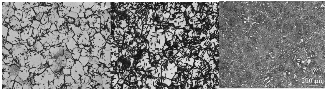
Fig.3 OM images of Ti-5321 alloy cooled at different rates: (a) 1 °C/min, (b) 0.5 °C/min, and (c) 0.25 °C/min
