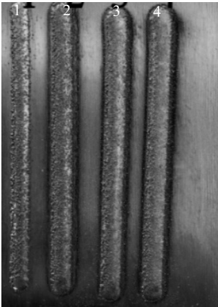
图 2 激光再制造工艺试样整体形貌 Fig.2 Overall morphology of laser remanufacture process samples
