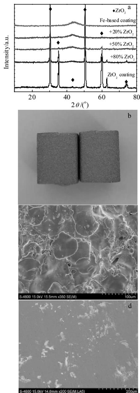
Fig.2 Phase structures and morphologies of coatings: (a) XRD patterns of sprayed coatings; (b) surface of sprayed coating; SEM morphology of composite coating with 20 wt%  $\text{ZrO}_2$ ; (c) original surface and (d) polished surface
