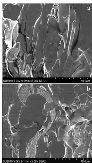
Fig.4 Bending fracture morphologies of the coatings: (a) metallic glassy coating and (b) composite coating with 20 wt% ZrO<sub>2</sub>
