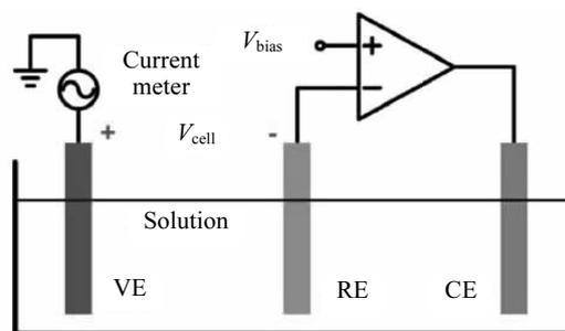
Fig.1 Diagram of the three-electrode system
