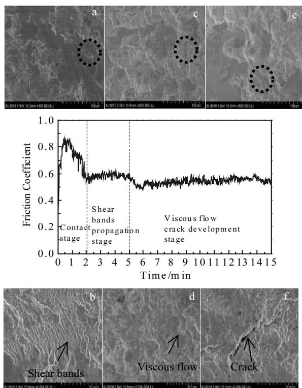
Fig.3 Friction coefficient value and worn surface morphologies of composite coating with 20 wt% ZrO<sub>2</sub> at 50 N load: (a) morphology of the coating after 3 min tribological test; (b) the magnified image of marked circle in Fig.3a; (c) morphology of the coating after 9 min tribological test; (d) the magnified image of marked circle in Fig.3c; (e) morphology of the coating after 15 min tribological test; (f) the magnified image of marked circle in Fig.3e
