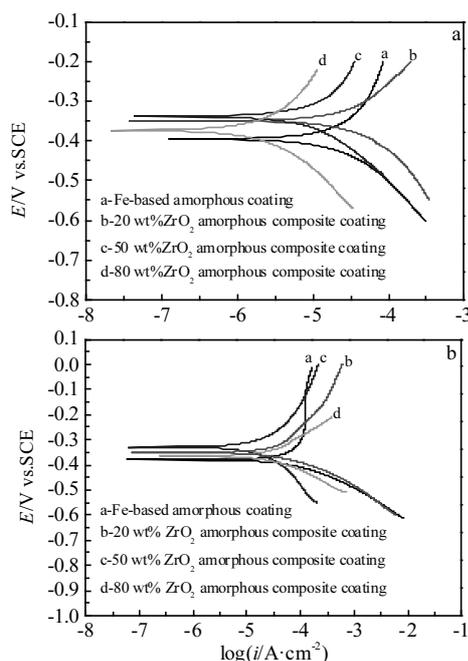
Fig.5 Potentiodynamic polarization curves of Fe-based glassy coating and composite coatings in 3.5 wt% NaCl solution (a) and 0.5 mol/L H<sub>2</sub>SO<sub>4</sub> solution (b)
