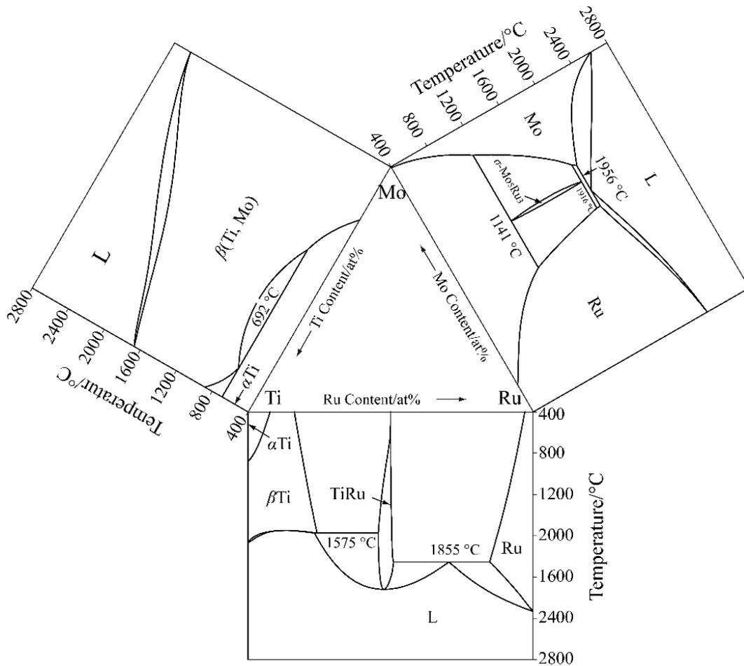
Fig.1 Binary phase diagrams constituting the Mo-Ru-Ti ternary system<sup>[11,20,26]</sup>
