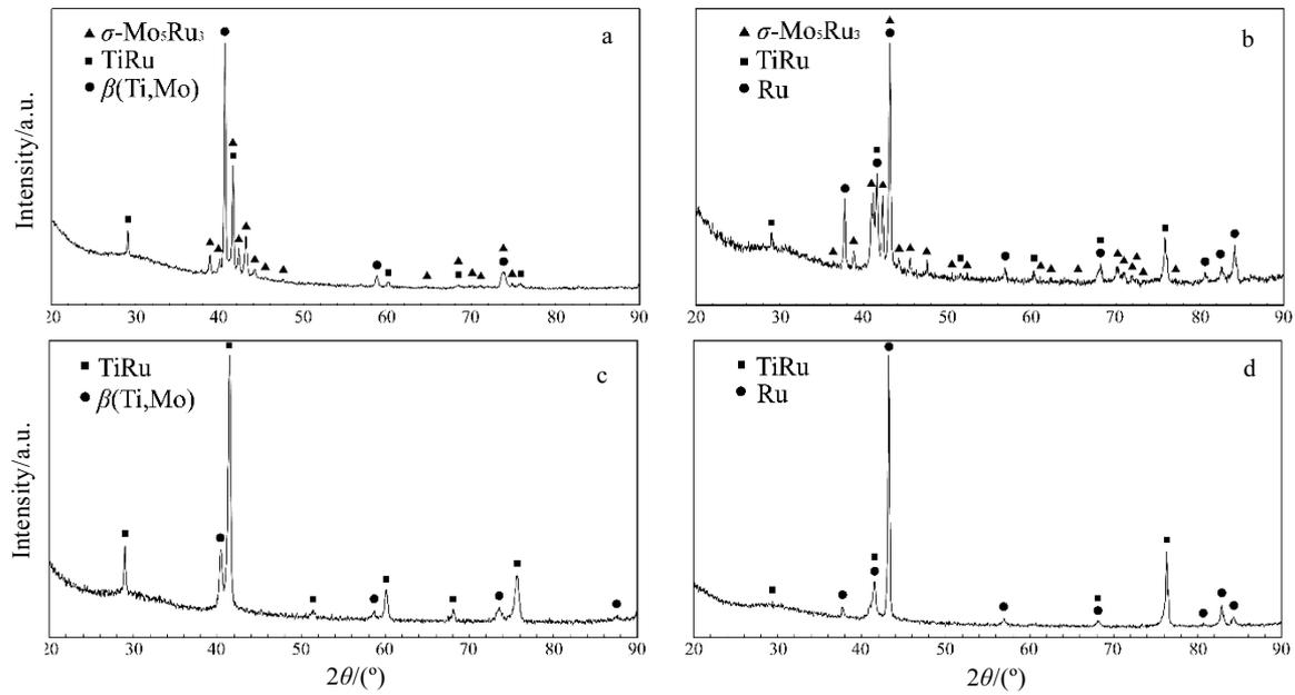
Fig.3 XRD patterns of ternary Mo-Ru-Ti alloys: (a)  $\text{Mo}_{55}\text{Ru}_{30}\text{Ti}_{15}$  alloy annealed at 1300 °C for 15 d, (b)  $\text{Mo}_{42}\text{Ru}_{51}\text{Ti}_7$  alloy annealed at 1100 °C for 50 d, (c)  $\text{Mo}_{15}\text{Ru}_{39}\text{Ti}_{46}$  alloy annealed at 1300 °C for 15 d, and (d)  $\text{Mo}_{15}\text{Ru}_{60}\text{Ti}_{25}$  alloy annealed at 1100 °C for 50 d
