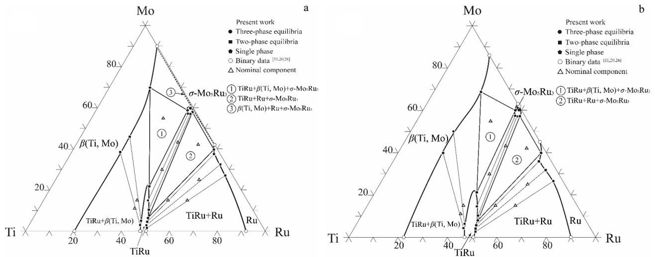
Fig.4 Experimentally determined isothermal section of Mo-Ru-Ti system at 1100 °C (a) and 1300 °C (b)
