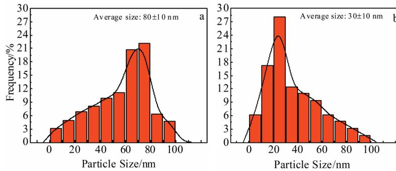
Fig.6 Particle size distribution of  $\theta'(Al_2Cu)$  participates in Al-Cu-Mn alloys with 0wt% (a) and 0.3wt% (b) Al-5Ti-0.8C master alloy
