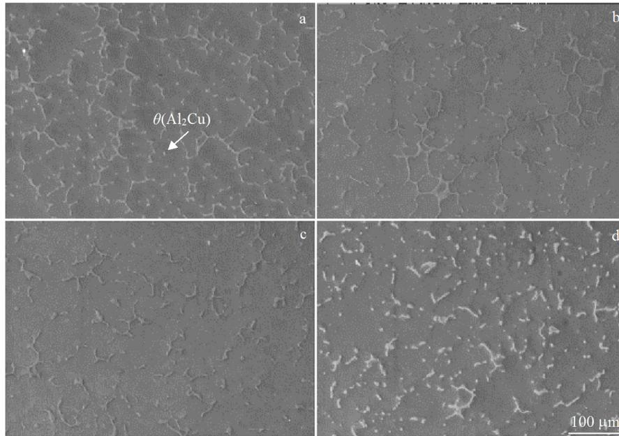
Fig.4 SEM images of Al-Cu-Mn alloy with different Al-5Ti-0.8C master alloy contents: (a) 0wt%, (b) 0.1wt%, (c) 0.3wt%, and (d) 0.5wt%
