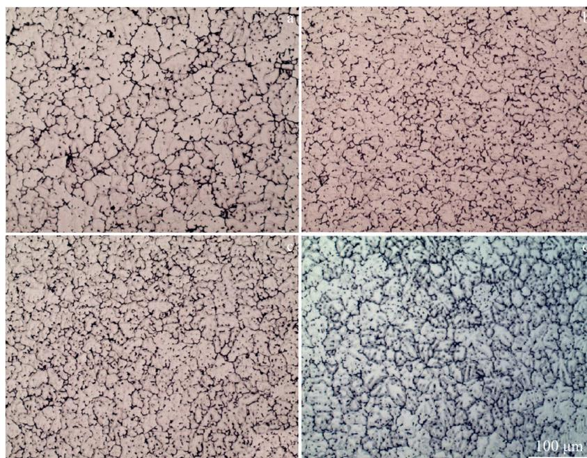
Fig.3 Microstructures of Al-Cu-Mn alloy with different Al-5Ti-0.8C master alloy contents: (a) 0wt%, (b) 0.1wt%, (c) 0.3wt%, and (d) 0.5wt%
