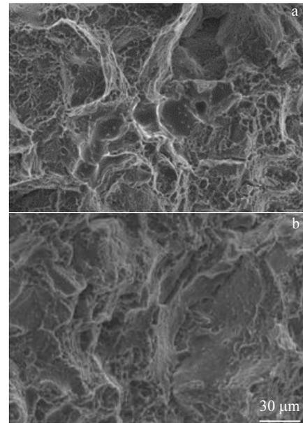
Fig.10 Tensile fractographies of Al-Cu-Mn alloy refined by different contents of Al-5Ti-0.8C master alloy: (a) 0wt% and (b) 0.3wt%
