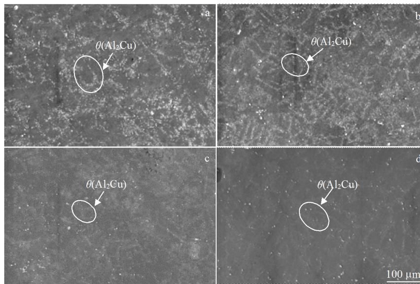
Fig.7 Microstructures of Al-Cu-Mn alloy refined by different contents of Al-5Ti-0.8C master alloy after heat treatment: (a) 0wt%, (b) 0.1wt%, (c) 0.3wt%, and (d) 0.5wt%
