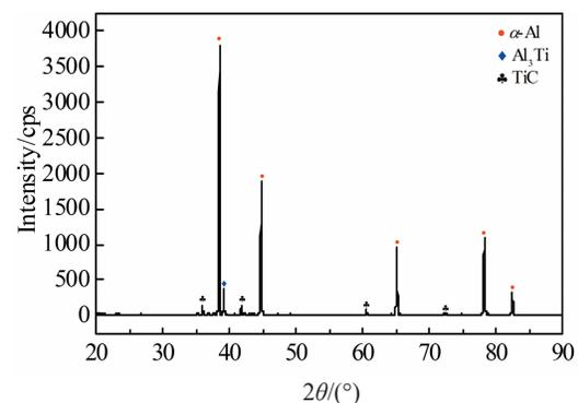
Fig.1 XRD pattern of Al-5Ti-0.8C master alloy
