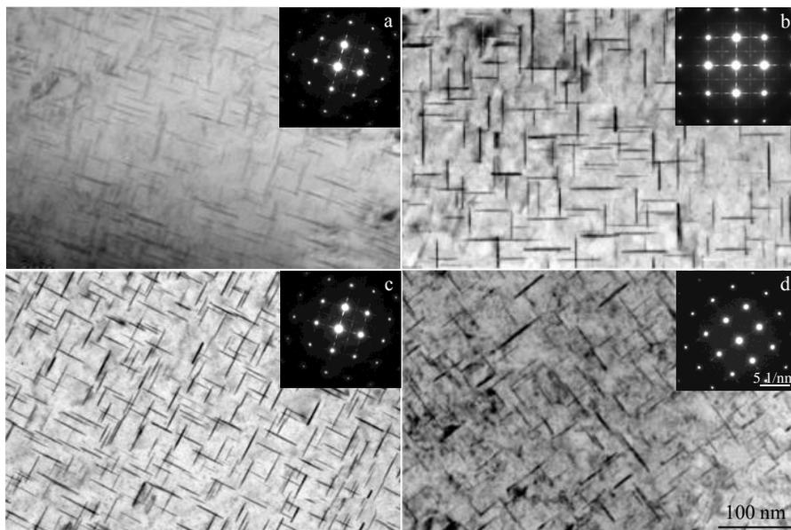
Fig.5 TEM images of Al-Cu-Mn alloy refined by different contents of Al-5Ti-0.8C master alloy after heat treatment: (a) 0wt%, (b) 0.1wt%, (c) 0.3wt%, and (d) 0.5wt%
