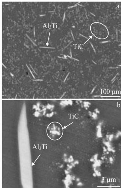
Fig.2 SEM images of Al-5Ti-0.8C master alloy at low (a) and high (b) magnification
