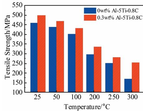
Fig.11 Tensile strength of Al-Cu-Mn alloy refined by 0wt% and 0.3wt% Al-5Ti-0.8C master alloy at elevated temperatures
