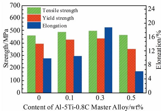
Fig.9 Tensile properties of Al-Cu-Mn alloys refined by different contents of Al-5Ti-0.8C master alloy after heat treatment
