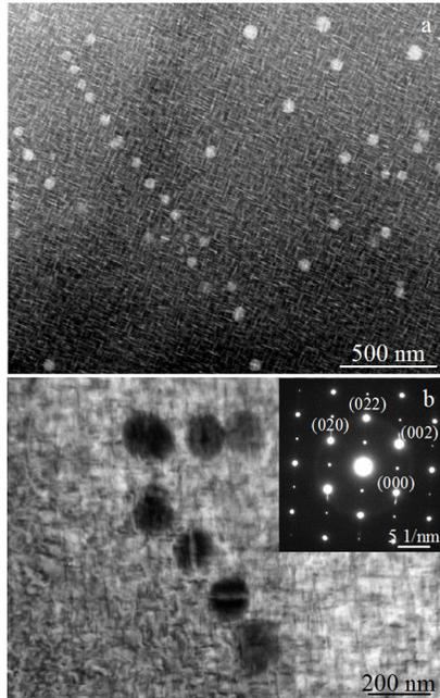
Fig.8 TEM images of  $\text{Al}_3(\text{Zr, Ti})$  phases at low (a) and high (b) magnification
