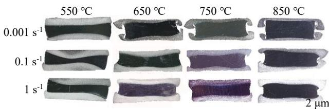
Fig.5 Macroscopic structures of TA1/N6/TA1 laminated composite under different conditions
