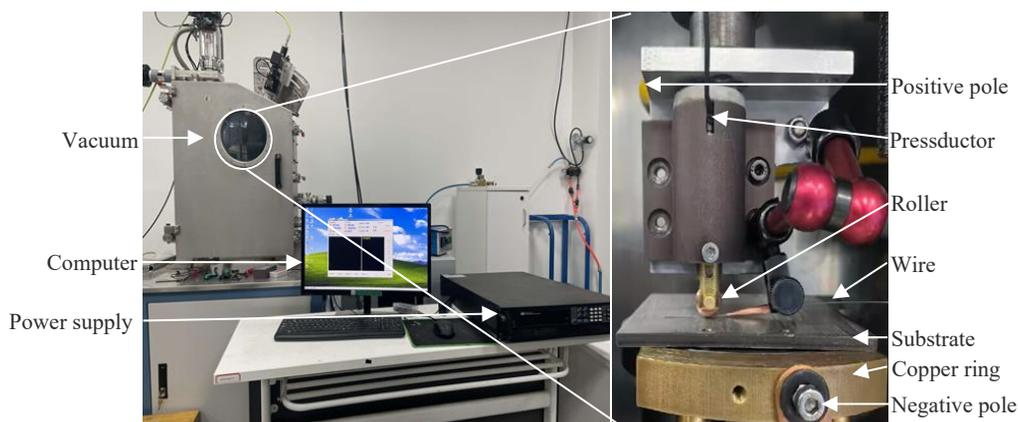
Fig.2 Equipment set of SP-JHAM process
