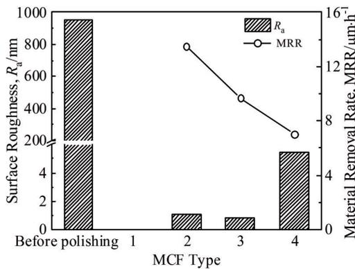
Fig.15 Surface roughness ( $R_a$ ) and MR rate (MRR) after scanning polishing for 60 min with different MCF slurries
