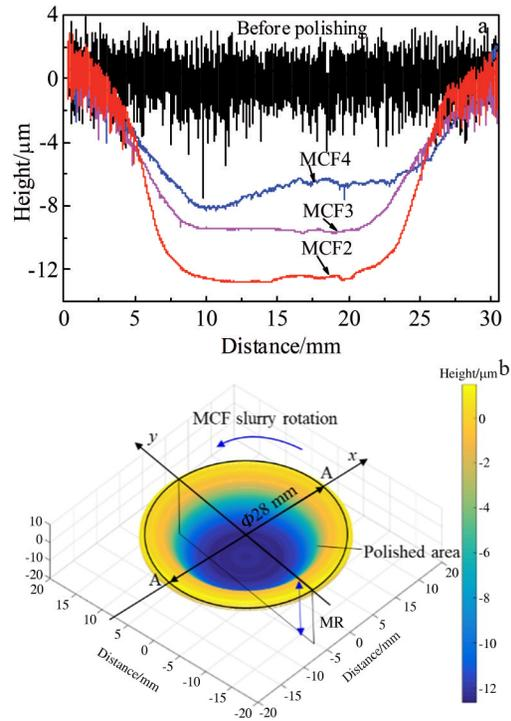
Fig.12 Cross-section profile (a) and 3D structure (b) of typical polished area after scanning polishing
