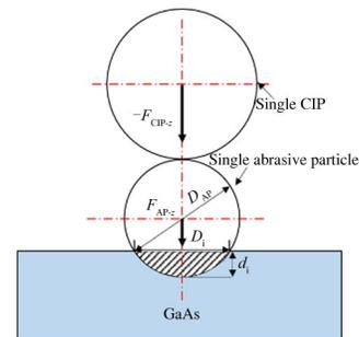
Fig.9 Schematic diagram of forces acting on CIP and abrasive particle under external magnetic field
