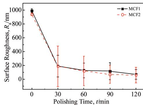
Fig.4 Surface roughness  $R_a$  of GaAs wafer after polishing by different MCF slurries for different durations
