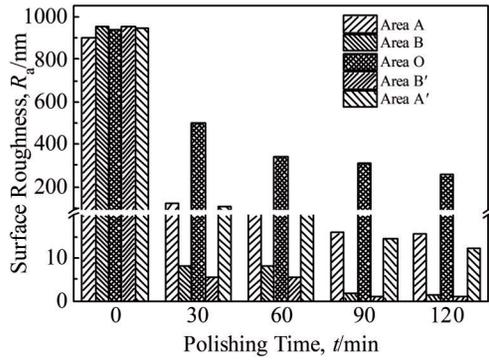
Fig.5 Surface roughness  $R_a$  at different areas on GaAs wafer after spot polishing by MCF2 slurry for different durations
