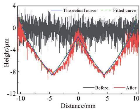
Fig.10 Experimental and simulated MR depth of GaAs wafer surface after polishing
