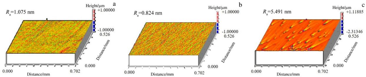
Fig.14 Surface morphologies at the center of polishing area after scanning polishing with MCF2 slurry (a), MCF3 slurry (b), and MCF4 slurry (c)
