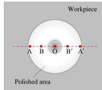
Fig.3 Schematic diagram of workpiece after MCF polishing for 60 min
