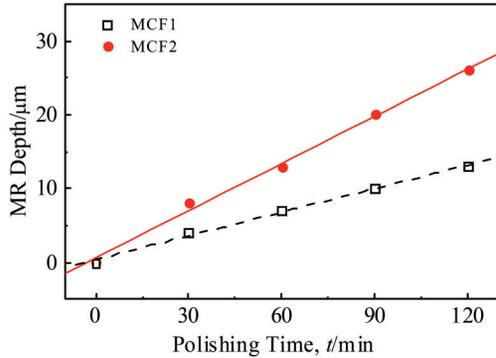
Fig.8 MR depth of wafer surface after spot polishing by MCF1 and MCF2 slurries for different durations
