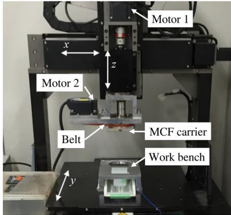
Fig.2 Appearance of experiment device
