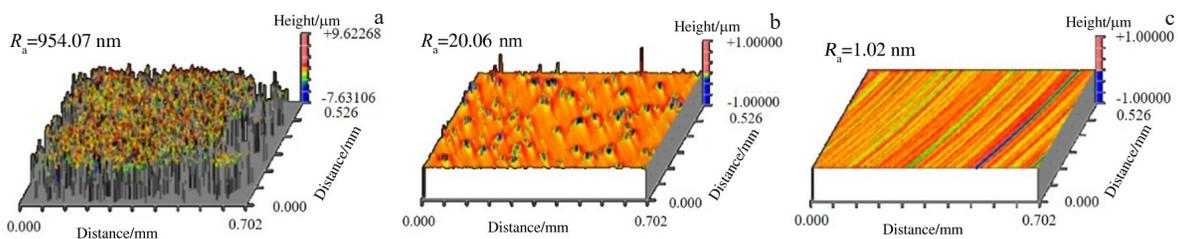
Fig.6 3D images of work surface before (a) and after spot polishing by MCF1 slurry (b) and MCF2 slurry (c)
