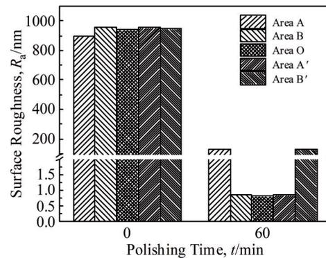
Fig.13 Surface roughness  $R_a$  at different areas on GaAs wafer after scanning polishing by MCF3 slurry for different durations
