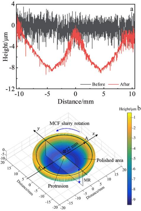
Fig.7 Cross-sectional profile (a) and 3D structure (b) of typical polished area after spot polishing by MCF2 slurry
