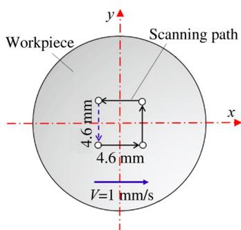
Fig.11 Schematic diagram of MCF polishing along scanning path
