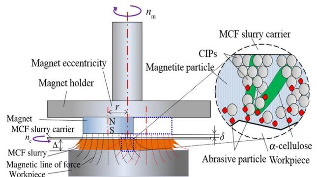
Fig.1 Schematic diagram of MCF polishing process
