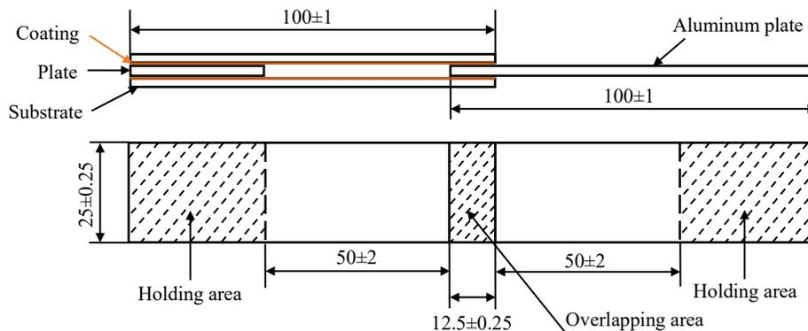
Fig.12 Schematic diagram of double lap shear strength test of  $Y_2O_3$ -PF alternating coating<sup>[24]</sup>
