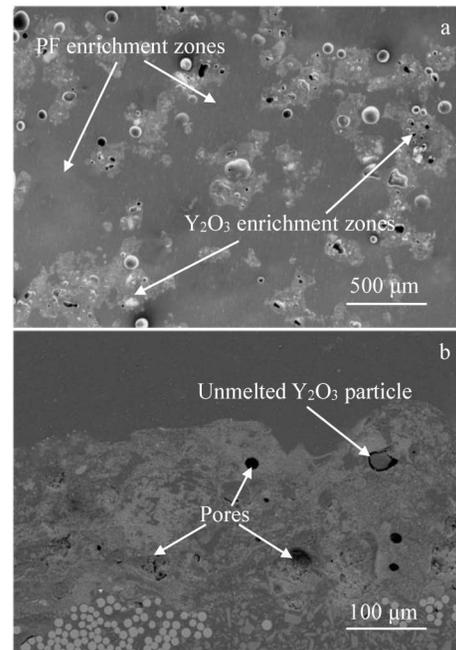
Fig.8 Microstructures of polished surface (a) and cross-section (b) of  $Y_2O_3$ /PF coating sprayed by external powder feeding
