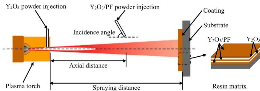
Fig.3 Schematic diagram of dual-channel supersonic plasma spraying process
