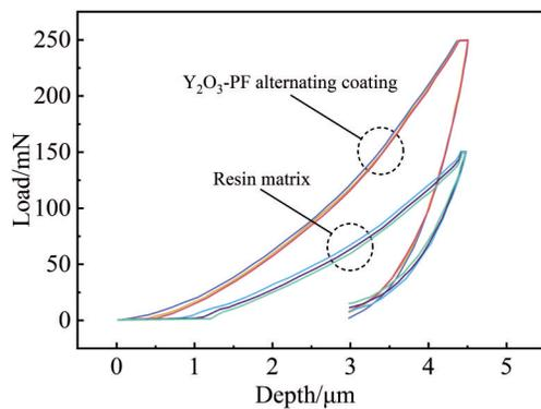
Fig.14 Load-depth curves of  $Y_2O_3$ -PF alternating coating and resin matrix
