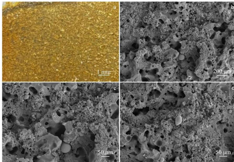
Fig.13 Peeling morphologies of  $Y_2O_3$ -PF alternating coating on aluminum plate after shear tests: (a) appearance; (b) SEM image at low magnitude; (c–d) SEM images at high magnitude
