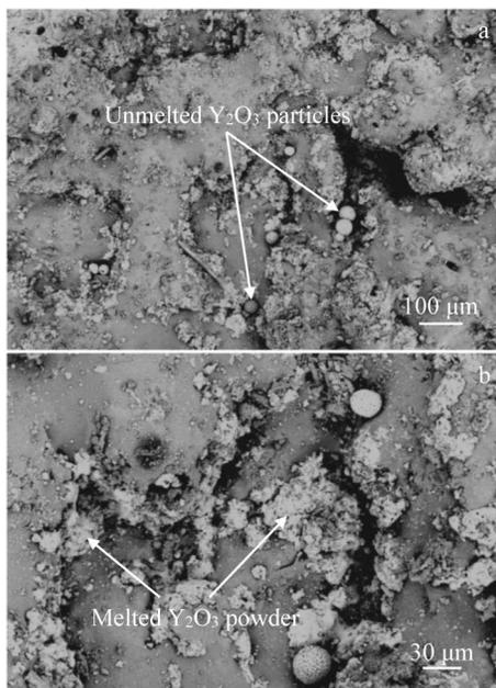
Fig.9 Surface morphologies of  $Y_2O_3$  coating sprayed by internal powder feeding at low (a) and high (b) magnitudes
