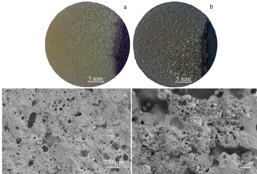
Fig.11 Appearances (a–b) and microstructures (c–d) of cross-sections of matrix (a, c) and  $Y_2O_3$ -PF alternating coating (b, d) after tensile fracture
