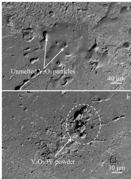
Fig.7 Spreading morphologies of  $Y_2O_3$ /PF coating sprayed by external powder feeding at low (a) and high (b) magnitudes
