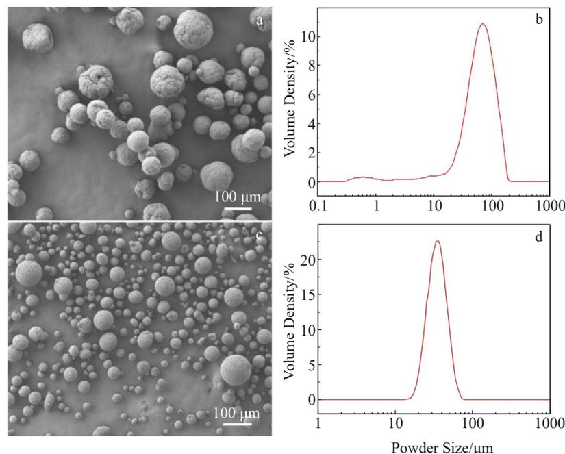
Fig.1 Surface morphologies (a, c) and particle size distributions (b, d) of  $Y_2O_3$ /PF composite powder (a–b) and  $Y_2O_3$  spherical powder (c–d)
