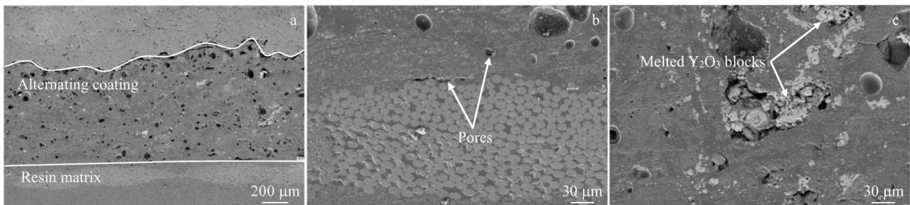
Fig.5 Cross-section morphologies of  $Y_2O_3$ -PF alternating coating at low (a) and high (b–c) magnitudes
