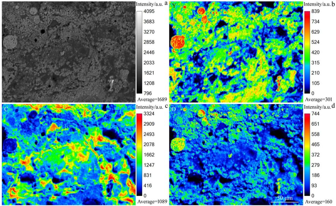
Fig.6 EPMA results of  $Y_2O_3$ -PF alternating coating: (a) overall morphology; (b) Y element mapping; (c) C element mapping; (d) O element mapping
