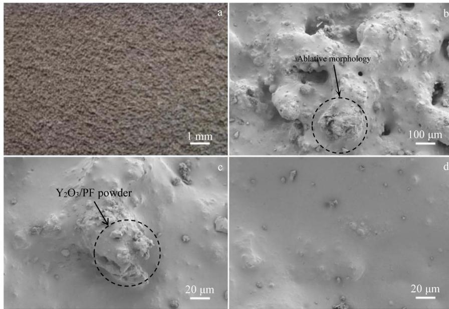
Fig.4 Appearance (a) and SEM morphologies at low magnitude (b) and high magnitude (c–d) of  $Y_2O_3$ -PF alternating coating surface
