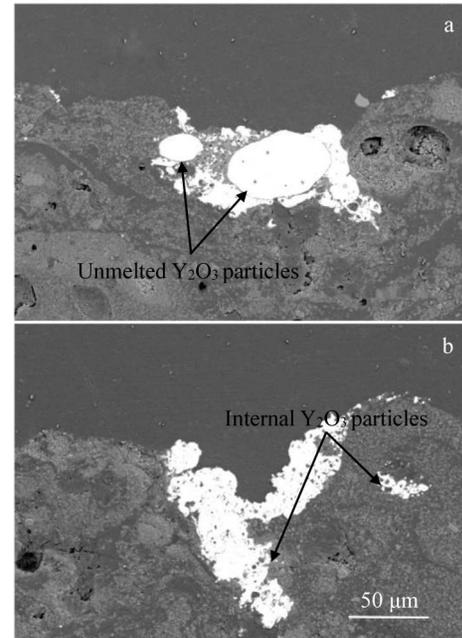
Fig.10 High-resolution cross-section morphologies of  $Y_2O_3$  coating: (a) unmelted  $Y_2O_3$  particles and (b) internal  $Y_2O_3$  particles
