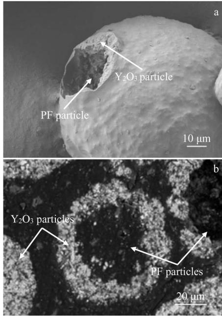
Fig.2 Surface (a) and cross-section (b) morphologies of  $Y_2O_3$ /PF composite powder
