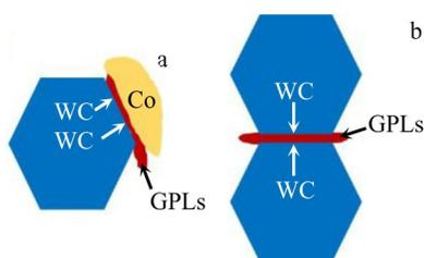
Fig.7 Schematic diagrams of GPLs distributed between WC/Co grain boundaries (a), and WC/WC grain boundaries (b)
