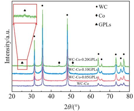
Fig.3 XRD patterns of WC-Co- $x$ GPLs cemented carbides
