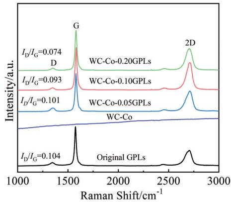
Fig.2 Raman spectra of original GPLs powder and WC-Co- $x$ GPLs powder mixtures ( $x=0.05\text{wt}\%$ ,  $0.10\text{wt}\%$ ,  $0.20\text{wt}\%$ )
