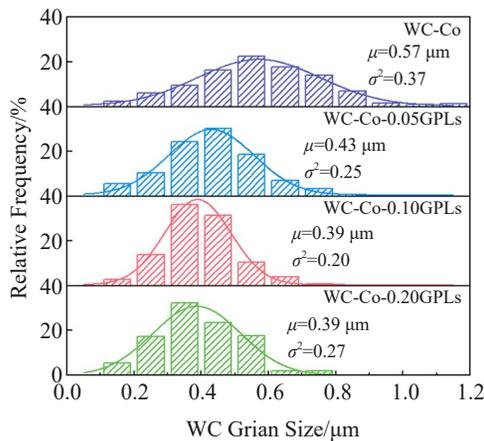
Fig.5 WC grain size distribution in WC-Co-xGPLs cemented carbides
