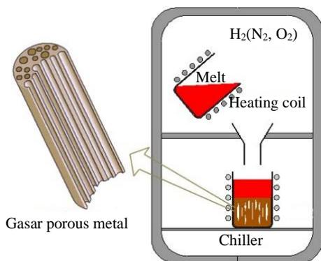
Fig.1 Schematic drawing of the mould casting apparatus
