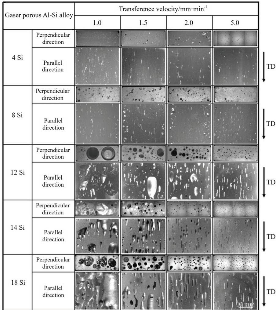
Fig.9 Specimens of Gasar porous Al-Si alloys fabricated by the continuous casting technology<sup>[20]</sup>
