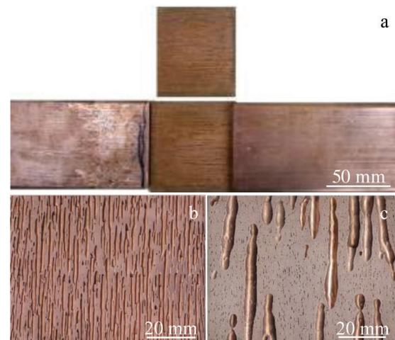
Fig.10 Mass production of Gasar porous Cu-6Zn (a) and Cu-6Ni (b) alloys fabricated by the continuous casting technique<sup>[29]</sup>
