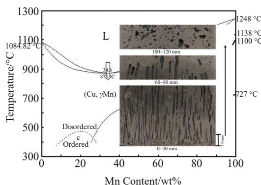
Fig.4 Cu-Mn equilibrium phase diagram and pore morphology of Gasar porous Cu-34.6%Mn alloy<sup>[17]</sup>
