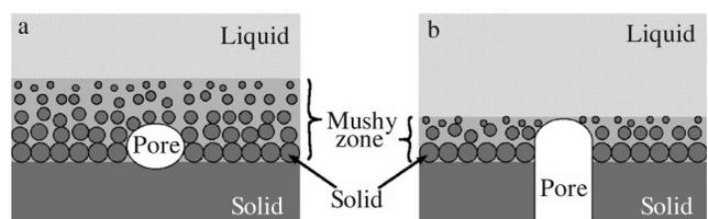
Fig.3 Mechanism of wide (a) and narrow (b) width of mushy zone influencing pore growth of Gasar porous Mg alloys<sup>[18]</sup>
