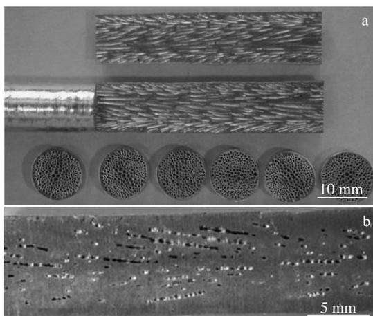
Fig.7 Specimens of Gasar porous stainless steel (a) and carbon steel (b) fabricated by the continuous zone melting technology<sup>[25,26]</sup>
