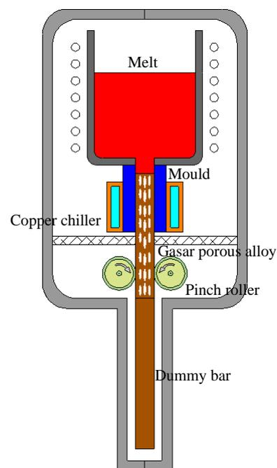
Fig.8 Schematic drawing of continuous casting apparatus
