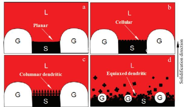
Fig.5 Morphologies of pores with different solidification modes: (a) planar, (b) cellular, (c) columnar dendrite, and (d) equiaxed dendrite<sup>[19]</sup>
