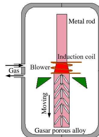
Fig.6 Schematic drawing of continuous zone melting technology
