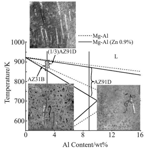
Fig.2 Effect of the width of mushy zone on pore morphology of Gasar porous Mg-Al alloys made by the mold casting technique<sup>[18]</sup>
