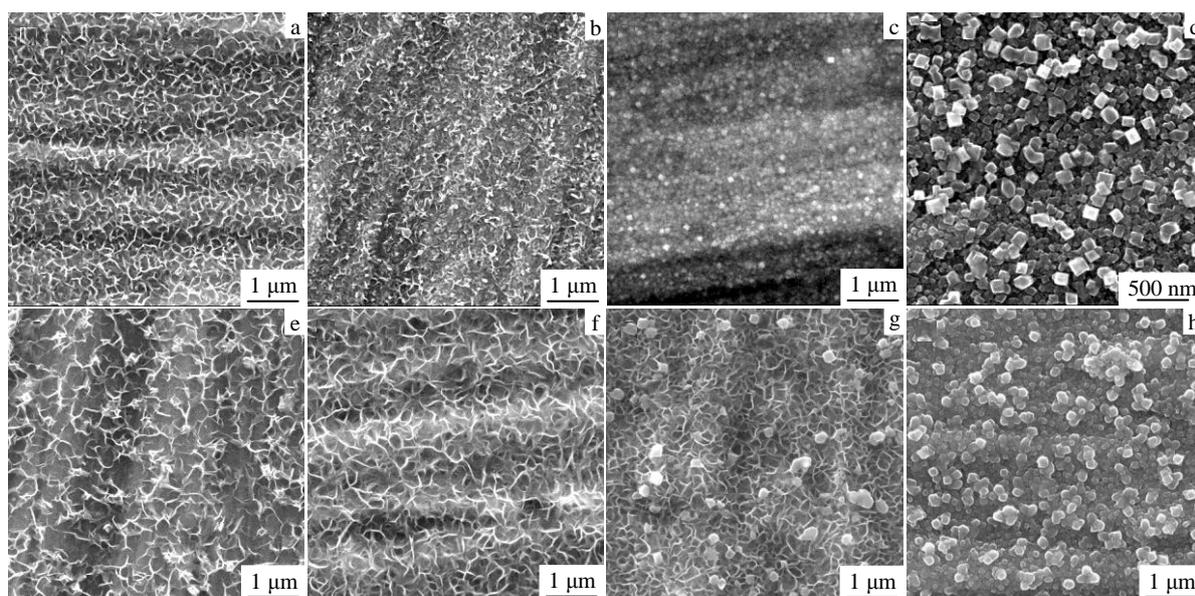
Fig.1 SEM images of the TLM alloy and Ti samples hydrothermally treated at different temperatures: Ti: (a) 105 °C, (b) 120 °C, (c) 150 °C, (d) 170 °C; TLM: (e) 105 °C, (f) 120 °C, (g) 135 °C, and (h) 150 °C
