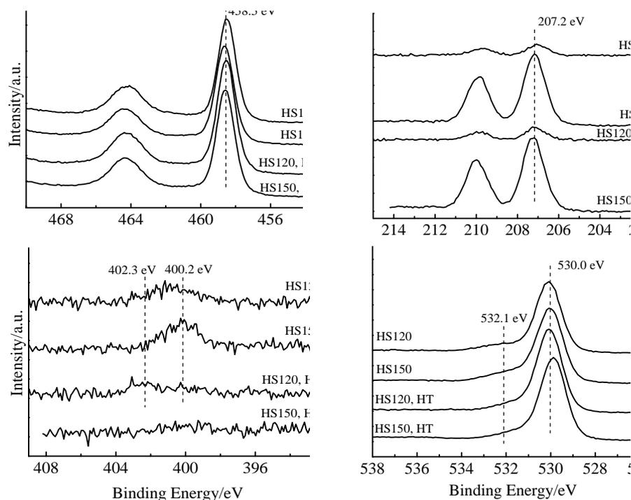
Fig.3 XPS spectra of the hydrothermally treated (HS) and the heat treated (HT) TLM alloy samples: (a) Ti 2p, (b) Nb 3d, (c) N 1s, and (d) O 1s
