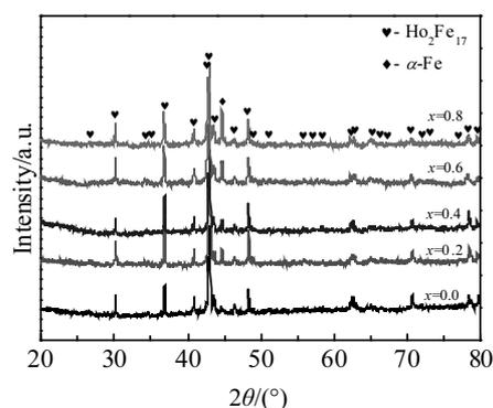
Fig.1 XRD patterns of  $\text{La}_x\text{Ho}_{2-x}\text{Fe}_{17}$  alloys
