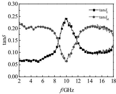
Fig.5 Relationship between loss tangent of La<sub>0.2</sub>Ho<sub>1.8</sub>Fe<sub>17</sub> powders and frequency
