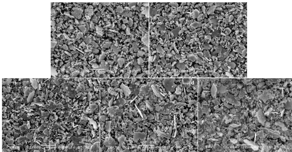
Fig.2 SEM images of the  $\text{La}_x\text{Ho}_{2-x}\text{Fe}_{17}$  powders: (a)  $x=0.0$ , (b)  $x=0.2$ , (c)  $x=0.4$ , (d)  $x=0.6$ , and (e)  $x=0.8$
