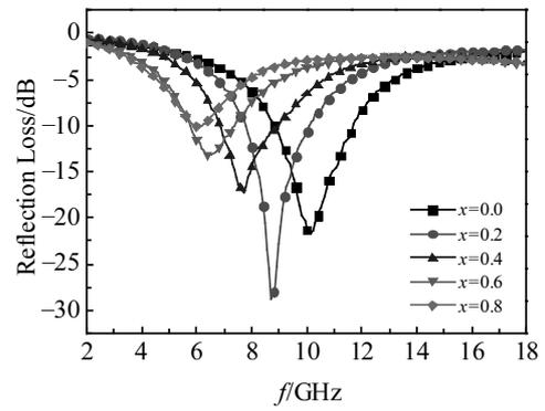
Fig.6 Reflection loss of the La<sub>x</sub>Ho<sub>2-x</sub>Fe<sub>17</sub> powders ( $d=1.8$  mm)
