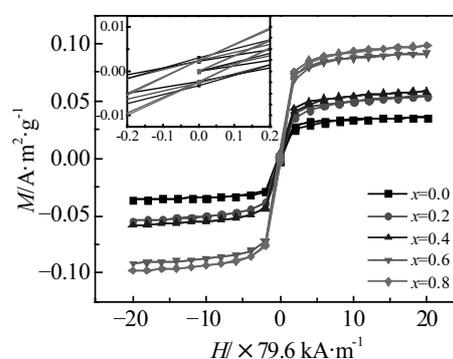
Fig.3 Magnetic hysteresis loops of the  $\text{La}_x\text{Ho}_{2-x}\text{Fe}_{17}$  powders
