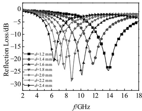
Fig.7 Reflection loss of the  $\text{La}_{0.2}\text{Ho}_{1.8}\text{Fe}_{17}$  powder with different thicknesses
