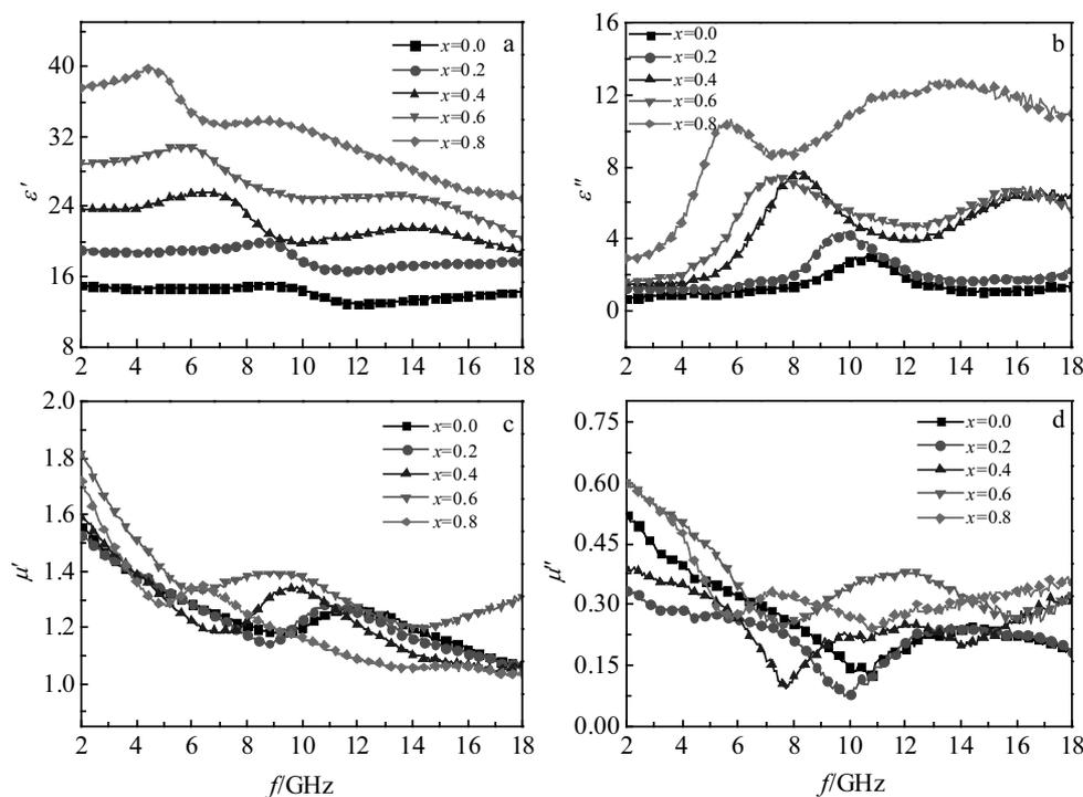
Fig.4 Electromagnetic parameters of  $\text{La}_x\text{Ho}_{2-x}\text{Fe}_{17}$  powders with the frequency variation: (a)  $\epsilon'$ , (b)  $\epsilon''$ , (c)  $\mu'$ , and (d)  $\mu''$
