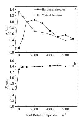
Fig.4 Relationship between surface roughness and tool rotation speed: (a) contact surface (values in horizontal and vertical directions) and (b) non-contact surface (average values of horizontal and vertical directions)
