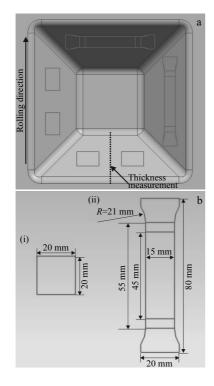
Fig.2 Sketch of test samples obtained by wire electrical discharge machining: (a) locations of the obtained samples and (b) geometrical dimensions of samples (i: surface quality and micro-hardness, ii: tensile test)
