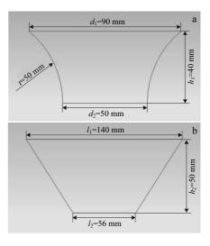
Fig.1 Geometrical details of designed parts: (a) truncated funnel and (b) pyramid frustum
