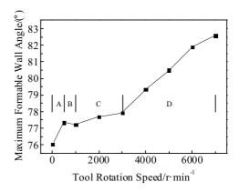
Fig.3 Formability at different tool rotation speeds
