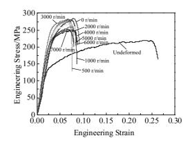
Fig.8 Engineering stress-strain curves of AA7075-O sheets at various rotation speeds
