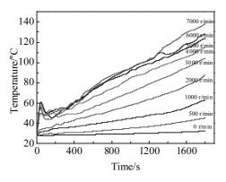
Fig.6 Temperature trends of AA7075-O sheets at different tool rotation speeds
