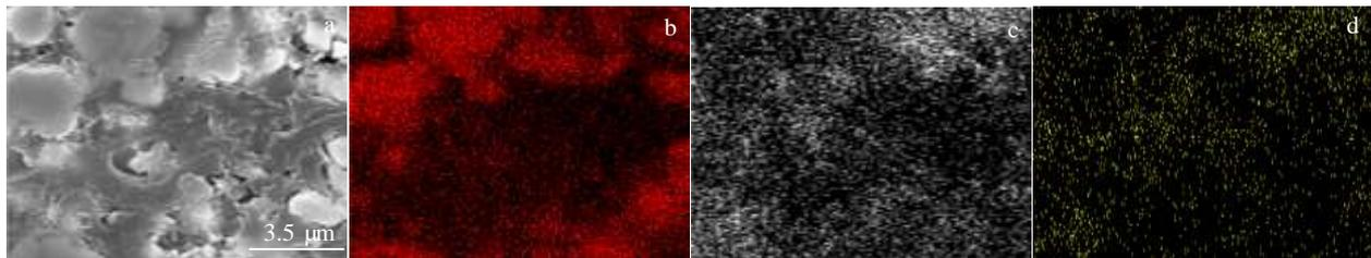
Fig.12 Cross section morphology of center region after ablation for 30 s (a) and elements distribution of Zr (b), Si (c), and Ta (d)
