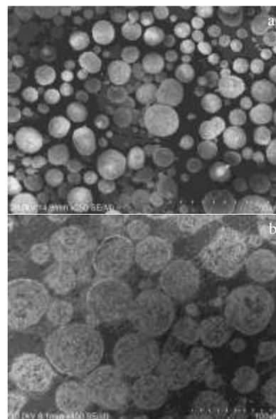
Fig.1 Morphologies of composite powder: (a) surface and (b) cross-section
