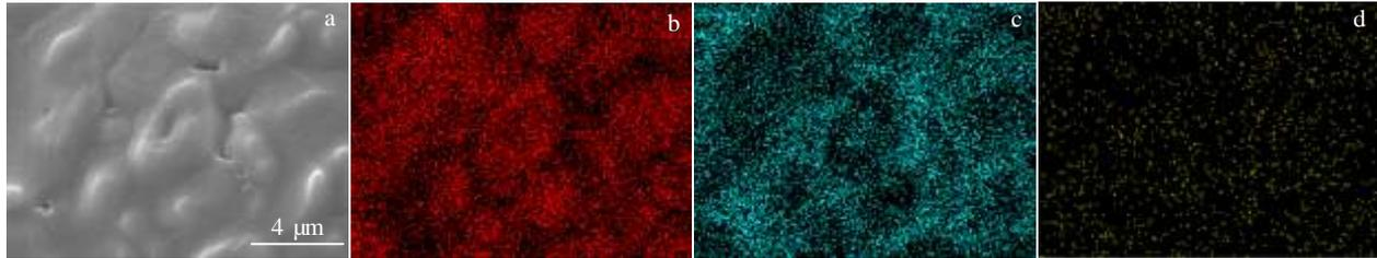
Fig.11 Morphology of center region after ablation for 30 s (a) and elements distribution of Zr (b), Si (c), and Ta (d)
