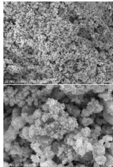
Fig.5 SEM surface morphology of coating (a) and its magnification (b)
