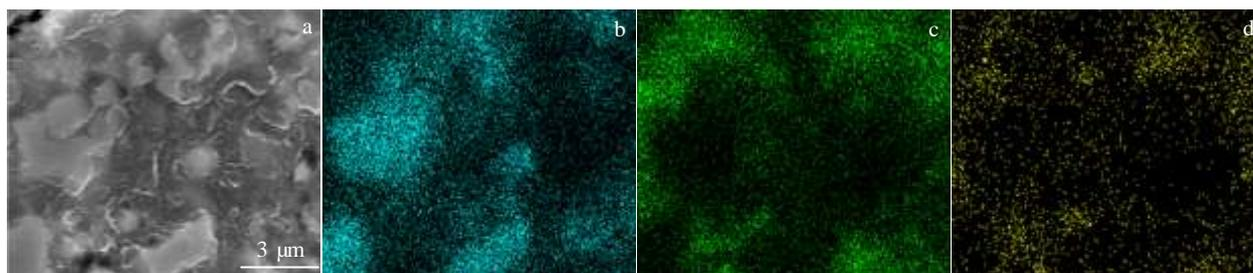
Fig.2 Morphology of cross-sectional composite powder (a) and element distribution of Zr (b), Si (c), and Ta (d)
