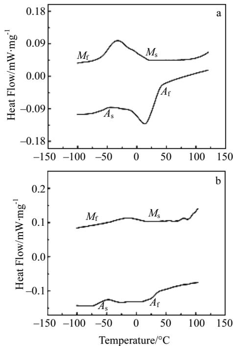
Fig.5 DSC curves of as-received NiTi particles (a) and NiTi<sub>p</sub>/WE43 composite (b) ( $A_s$  and  $A_f$  represent austenite start and finish points, respectively;  $M_s$  and  $M_f$  represent martensite start and finish points, respectively)
