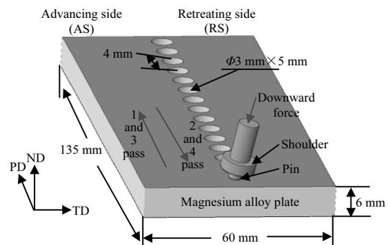
Fig.2 Schematic of FSP NiTi<sub>p</sub>/WE43 composite (PD, TD and ND represent processing, transverse and normal direction, respectively; AS of the plate is where the rotation speed of stir tool has the same direction as its travel speed; RS means that the two speed components have opposite directions)
