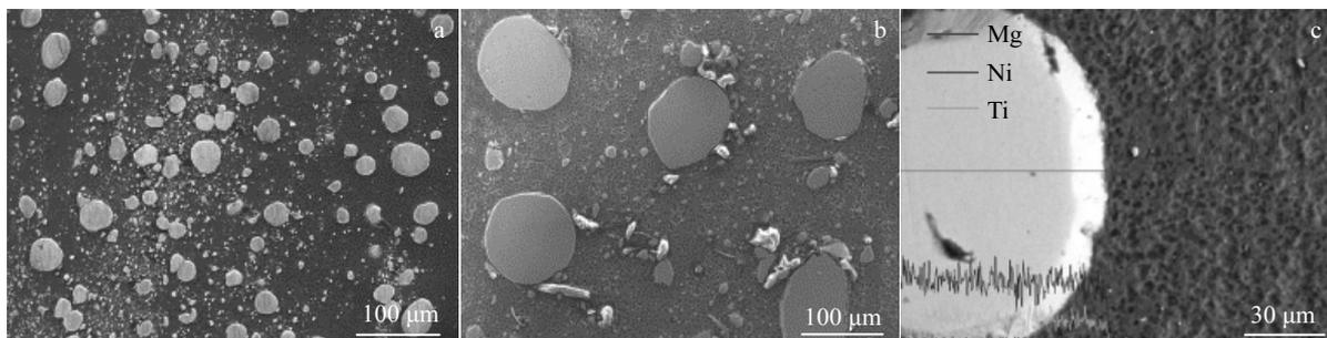
Fig.3 SEM images of the distribution of fine (a) and coarse (b) NiTi particles in NiTi<sub>p</sub>/WE43 composites; EDS results of the distribution of interfacial element between coarse NiTi particles and Mg matrix (c)
