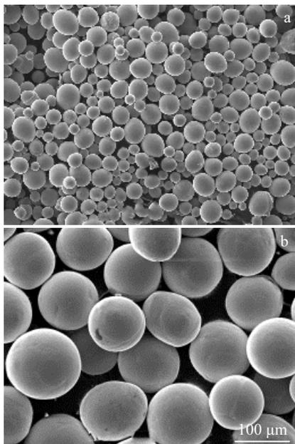
Fig.1 Morphologies of as-received fine (a) and coarse (b) NiTi particles
