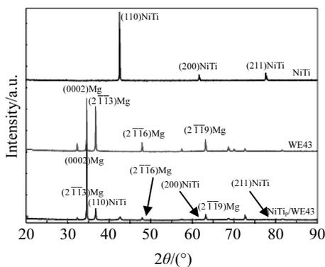
Fig.4 XRD patterns of as-received NiTi particles, WE43 Mg matrix and NiTi<sub>p</sub>/WE43 composite
