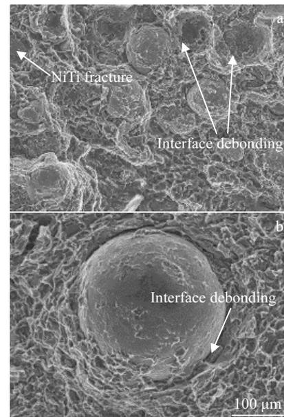
Fig.6 Fracture surfaces of NiTi<sub>p</sub>/WE43 composite with fine NiTi particles (a) and coarse NiTi particles (b)
