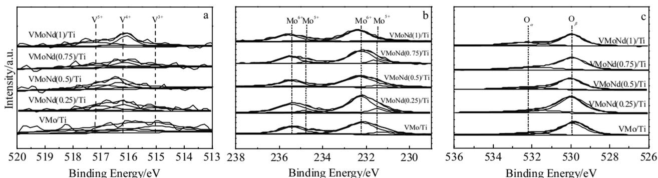
Fig.3 XPS spectra of V 2p (a), Mo 3d (b) and O 1s (c) of different catalysts
