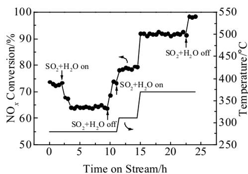
Fig.9 Effects of  $SO_2$  and  $H_2O$  on  $NO_x$  conversion for VMoNd(0.5)/Ti catalysts
