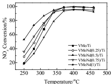
Fig.7  $NO_x$  conversion of different catalysts
