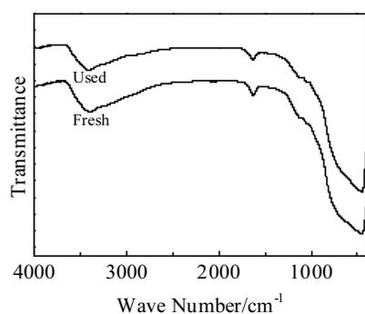
Fig.11 FT-IR spectra of fresh and used VMoNd(0.5)/Ti catalysts
