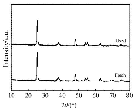
Fig.10 XRD patterns of fresh and used VMoNd(0.5)/Ti catalysts
