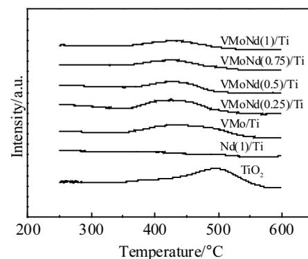
Fig.6 NH<sub>3</sub>-TPD profiles of different catalysts
