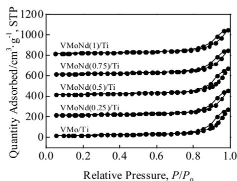
Fig.2  $\text{N}_2$  adsorption-desorption isotherms of different catalysts
