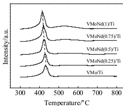
Fig.4 H<sub>2</sub>-TPR profiles of different catalysts
