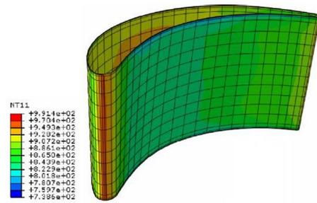
Fig.11 Temperature distribution of high temperature airflow in the vane area<sup>[28]</sup>
