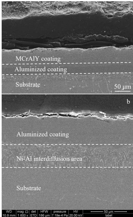
Fig.2 Aluminized coating+MCrAlY coating structure (a) and aluminized coating (b)
