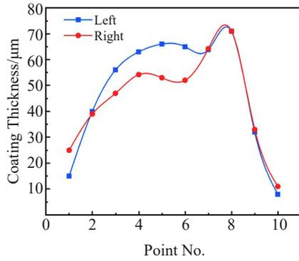
Fig.4 Variation curves of coating thickness on failed vanes
