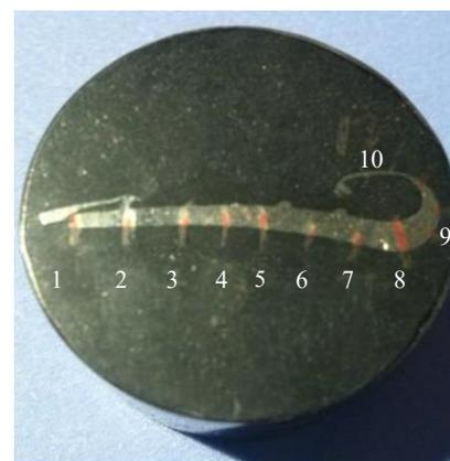
Fig.3 Inlaid vane specimen and its selected marking points
