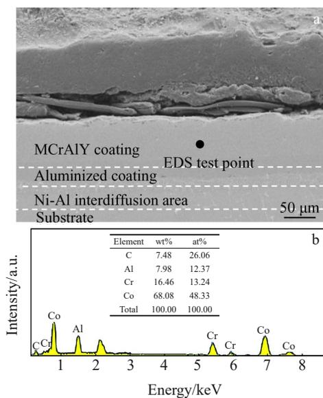
Fig.7 Micromorphology (a) and EDS analysis result (b) of MCrAlY coating in vane's basin area
