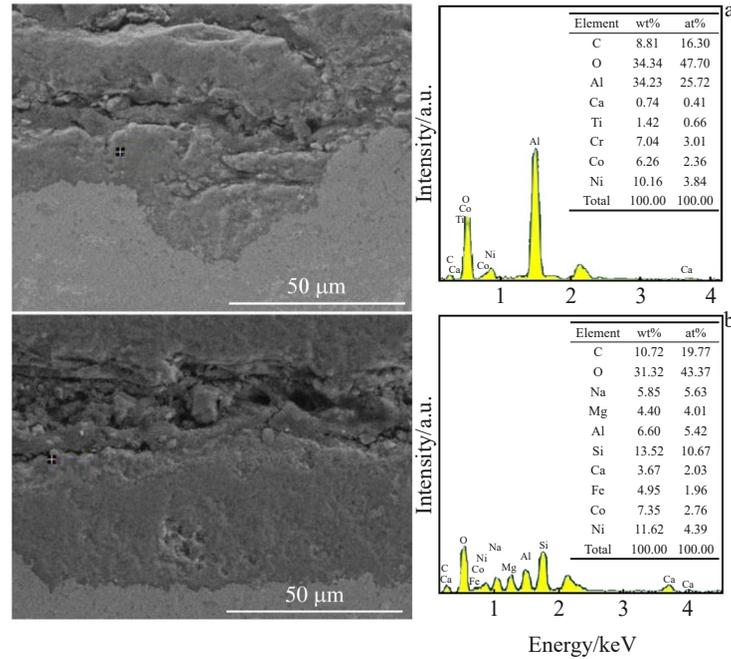
Fig.10 EDS analysis results of oxidation corrosion products on different surface areas of MCrAlY coating at the leading edge of the vane
