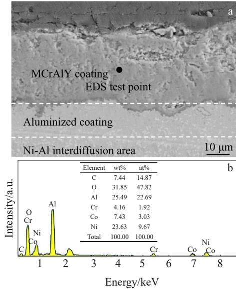
Fig.5 Micromorphology (a) and EDS analysis result (b) of MCrAlY coating on the trailing edge of the vane
