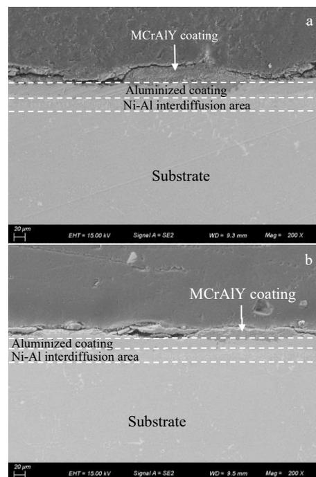
Fig.9 Micromorphologies of MCrAlY coating in different areas at point 10 of the leading edge of vane
