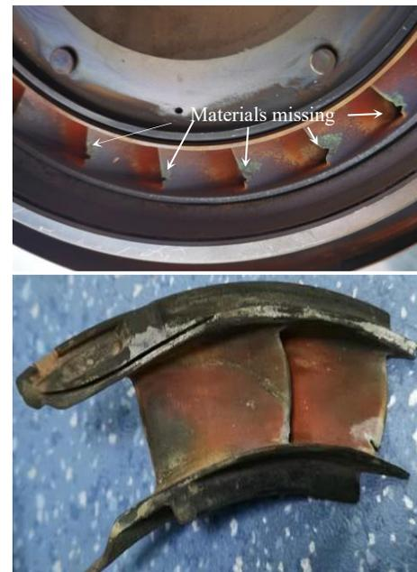
Fig.6 Material missing from the trailing edge of APU guide vane due to ablation
