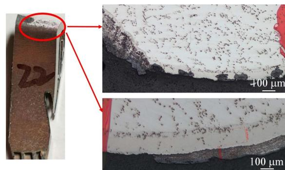
Fig.12 Coating thinning and spallation caused by CMAS corrosion-high temperature oxidation coupling effect
