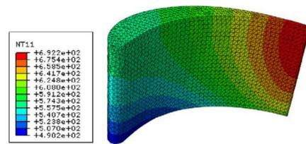
Fig.8 Temperature distribution of blade pressure surface when 1000 °C is applied for 200 s<sup>[28]</sup>
