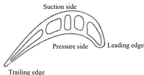
Fig.1 Schematic diagram of a certain type of APU high-pressure turbine guide vane
