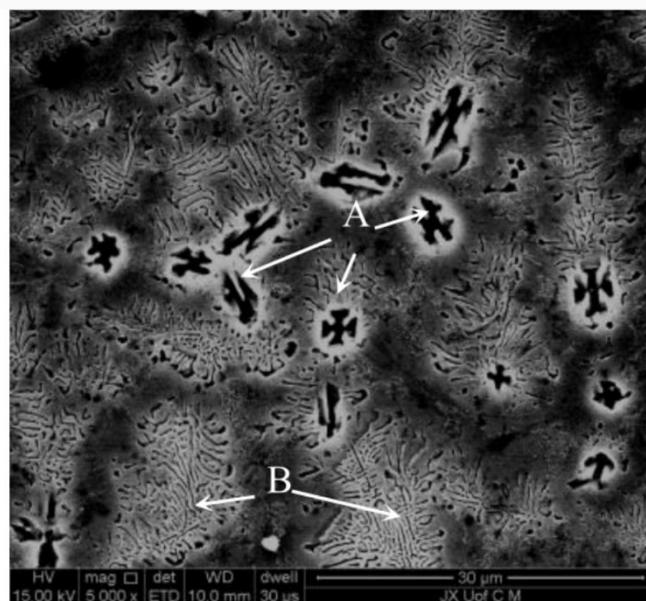
Fig.3 Microstructure of 15wt%Mg 2 Si/Al with laser power of 900 W
